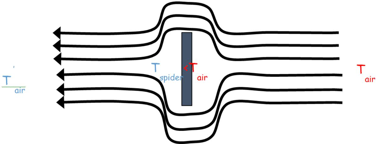
**Figure 2: Scenario of the LWE : the radiative transfer decreases the temperature of the spider. Some heat exchange exist between the air at temperature  $T_{air}$  and the spider, leading to a difference**
