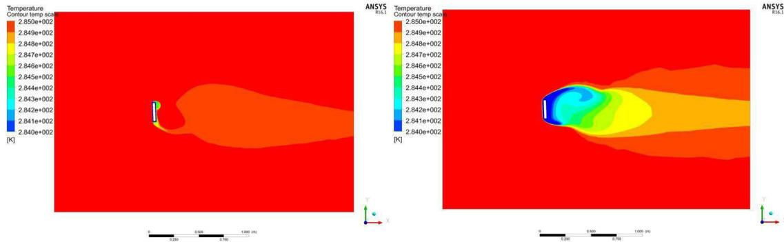
**Figure 3: ANSYS simulations results. The 2D temperature map in a vertical plane orthogonal to the spider direction is shown. Air flow is coming from the left, telescope is at the bottom.**
