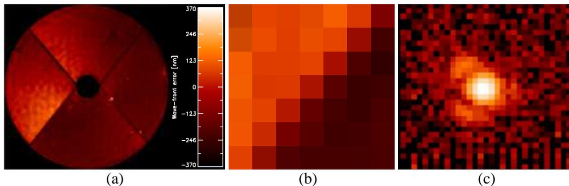
**Figure 1: Wave-front aberration measured by ZELDA WFS of SPHERE, during on-sky measurement of commissioning 4. (a) Measurement taken on the whole pupil. (b) Zoom of (a) on an area covered by one subaperture, along the spider arm bottom/left. The aberration presents strong discontinuities up to hundreds of nanometers (optical wave-front). (c) effect of LWE pattern in the focal plane of DTTS, H band imaging.**
