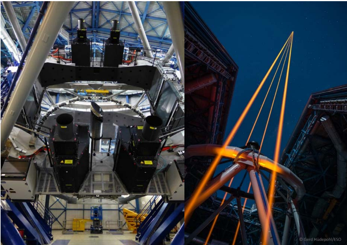
Figure 1 - Left: the four LGS Units mounted on the Yepun centerpiece with their respective laser and instrument control cabinets. Right: a view of a launch of the four lasers.
