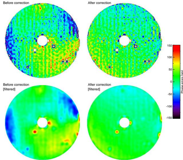
Figure 6. **Top:** Illustration of the ZELDA measured phase maps of the noncommon path aberrations (NCPA) on VLT/SPHERE using IRDIS before and after correction of these errors. **Bottom:** Same maps but filtered in Fourier map with a Hann window of size  $25 \lambda/D$  to avoid any spatial aliasing. Low spatial frequency aberrations are clearly visible on the left, while they have disappeared after the correction, except for a small amount of residual tip-tilt.
