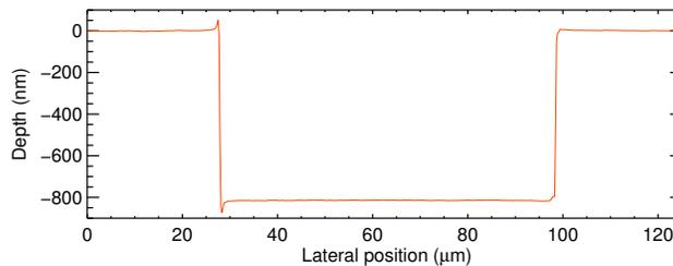
Figure 3. General profile of the phase mask measured by profilometry using a Wyko interference microscope. The mask presents measured depth and diameter  $70.7 \mu\text{m}$  and  $814.6 \text{ nm}$ , which are consistent to within 1% and 0.1% with the specifications and accuracy range of the process.
