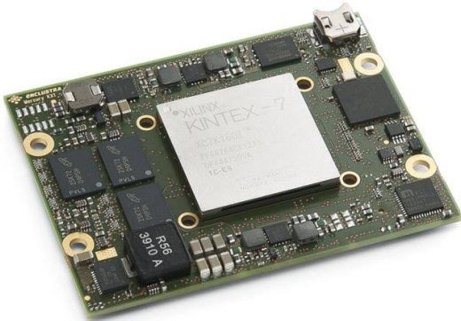
Figure 16: Enclustra FPGA board. Only 72×54 mm.
