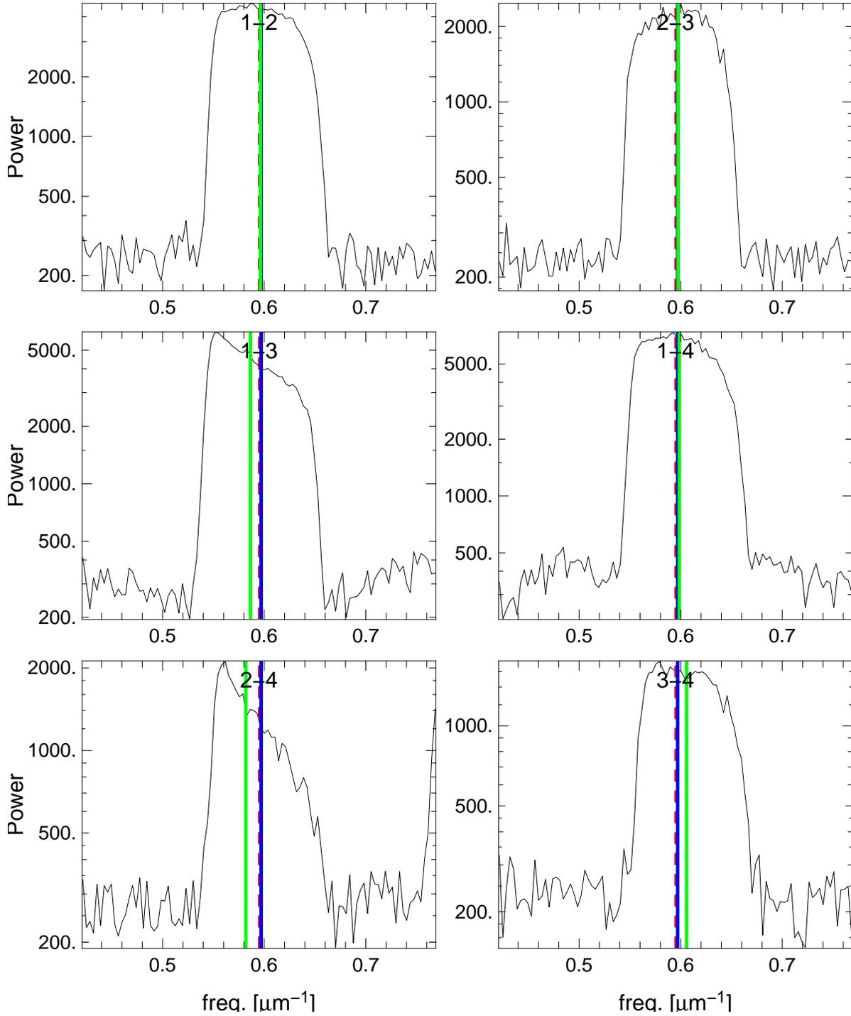
Figure 1. Band passes for the 6 baselines recorded in the FREE mode.
