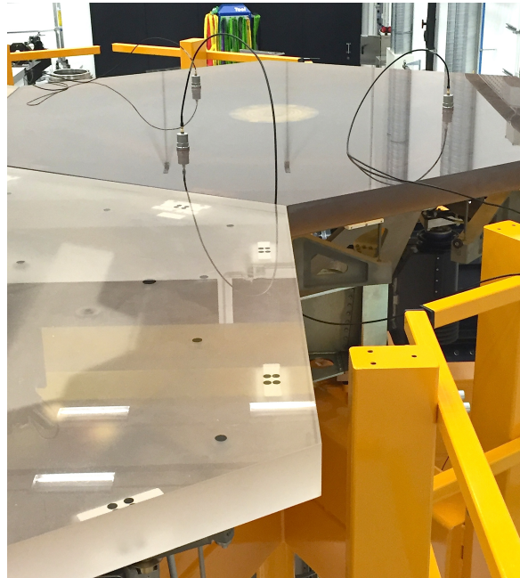
Figure 11. Accelerometers on the top of a segment in the M1 test facility with actuators using the active damping loop
