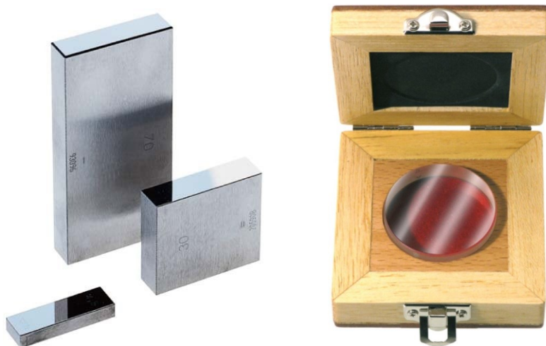
Figure 10 Precision gauge blocks (nominal thickness \pm 0.1 micron) and precision glass plate (high flatness of 0.125 micron) for calibration
