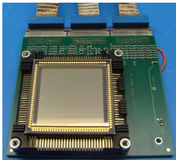
Figure 3b: AQUARIUS MUX mounted in its socket
