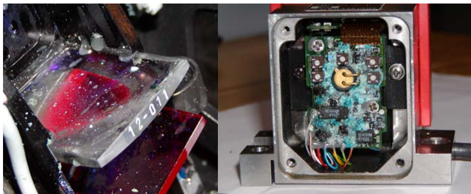
Figure 6. These pictures show some optical components and the damaged encoder head.
