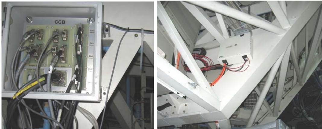
Figure 15 New junction boxes were installed inside of the M1 cell to avoid getting access to LCU, that was difficult and slow, an important reduction of time dismounting the Cassegrain adapter rotator was achieved thanks to this improvement.
