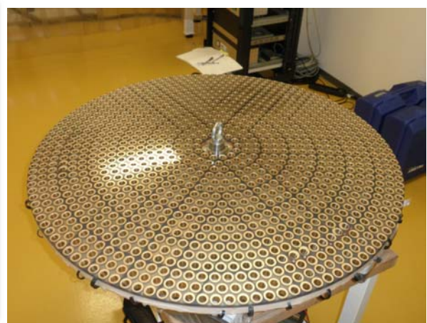
Figure 3: The DSM reference body manufactured by SESO ((left). On the right-hand side the reference body after coating; one sees the metallic rings realizing the capacitance with the back coating on the shell for gap measurement.
