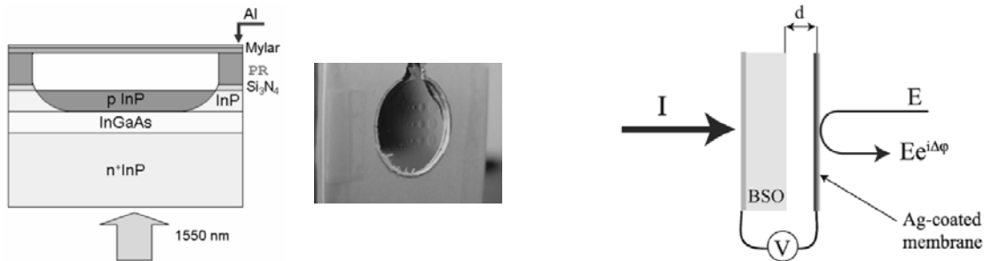
Figure 6. Optically addressed DMs concepts. Left (extracted from [15]): an InGaAs photodetector is coupled to a micromachined thin membrane mirror; a picture of a multi-detector prototype is represented, each detector having a different diameter. Right (extracted from [16]): a photorefractive BSO crystal is coupled to a micromachined thin membrane mirror; a bias AC voltage is applied across the DM; illumination spatial variations convert into spatial control of the membrane deflections.
