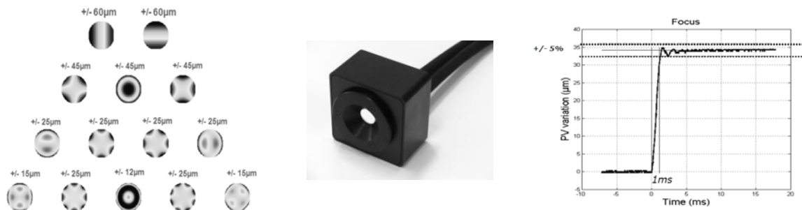
Figure 14. ALPAO DM features. Left: stroke vs correction mode, expressed in wavefront amplitude (DM277-15). Center: picture of an ALPAO DM. Right: response time characterization
