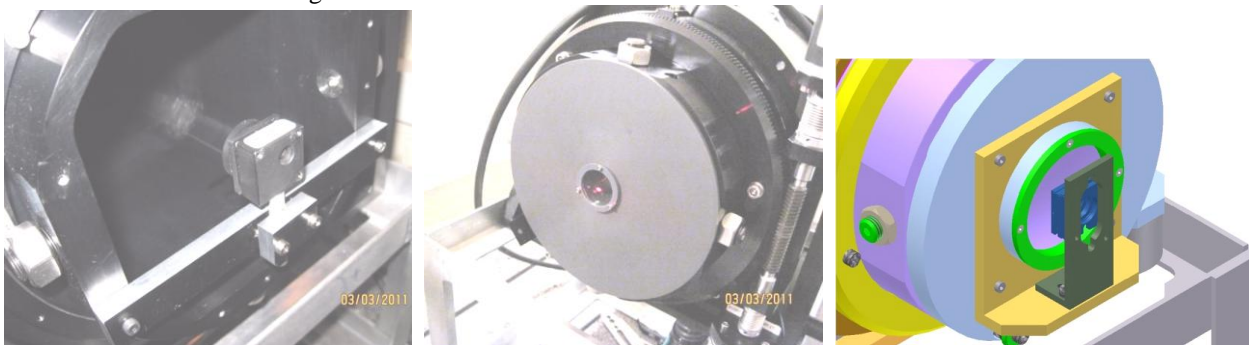
Figure 8: Left: Alignment mirror of ODM. Middle: Alignment target of ODM. Right: Alignment target of OD
