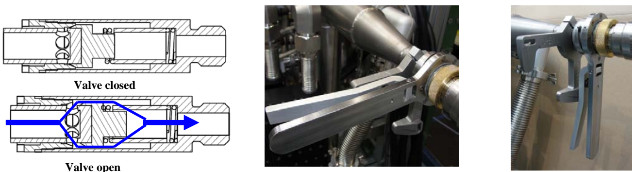
Figure 3: Main connection valve system
