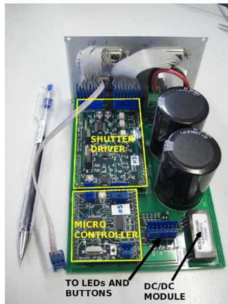
Figure 8: Mother board with microcontroller and shutter driver board
