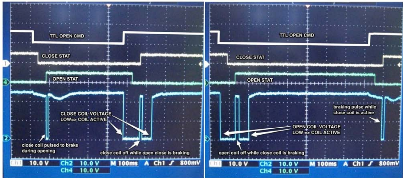
Figure 9: SDCU coil and status signal for braking mode
