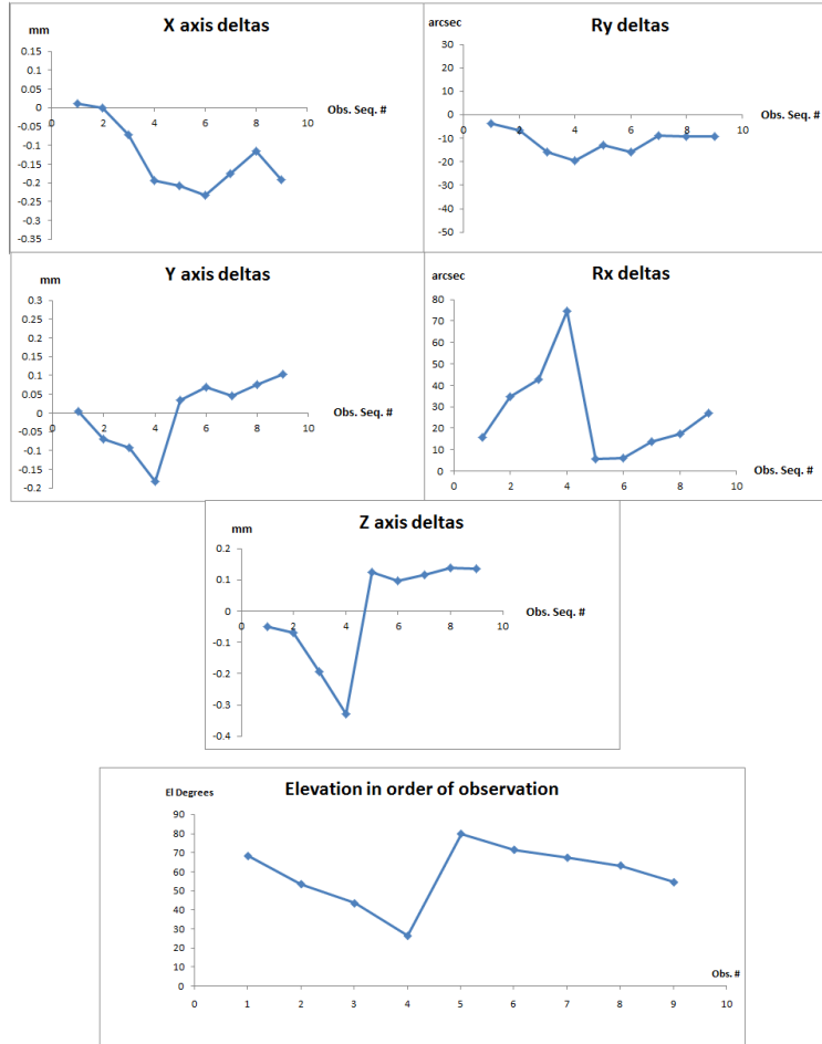
Figure 5. Plotted here are the same axis-error data as in figure 4, but this time vs. order of observation. Obviously the sudden jumps in Y, Rx and Z are related to a jump in elevation, (as shown also by the linearity for these errors in figure 4), but also there is some small drift at about the same level shown with the LBC data in figure 3.
