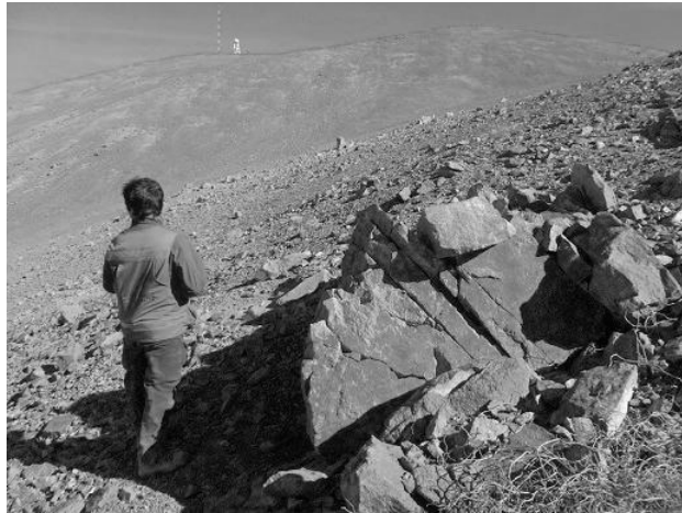
Picture 3-2 Photograph of a granitoid outcrop, showing slightly weathered discontinuity surfaces.
