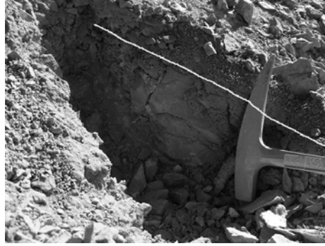
Picture 3-4: Example of the reduced soil cover on the rocks found at the hillside. The white line shows the contact between both materials.
