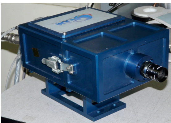
Figure 4. Left: Close-up photo of the OCam camera. Sub-electron noise has been demonstrated. Right: Image of OCam team (Left to right: Christian Guillaume, Jean-Luc GACH, Philippe Feautrier, and Philippe Balard) taken by the OCam camera with CCD220 cold and with L3Vision multiplication gain.
