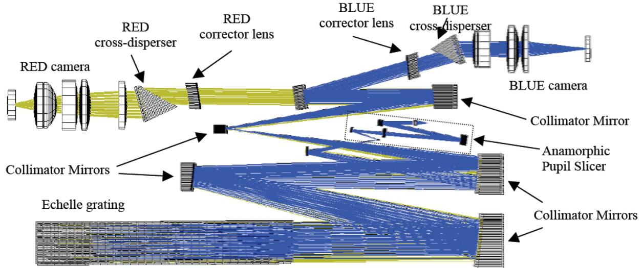
Figure 1. Optical layout of the ESPRESSO spectrograph
