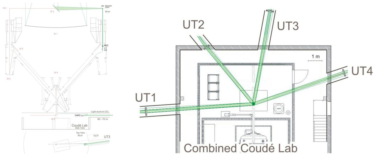
Figure 3. Left: Optical path from the M3 of an Unit Telescope (UT) of the VLT to the entrance of the light tunnels. Right: Incoherent recombination of the light beams from the four UTs in the Combined Coudé Laboratory, before being injected into a single spectrograph fiber.
