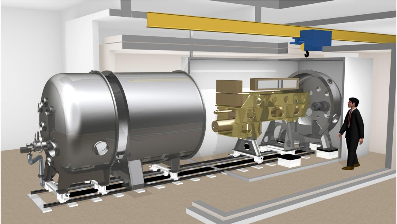
Figure 5. Mechanical layout showing the open vacuum vessel and the spectrograph, as well as a sketch of the thermal enclosure
