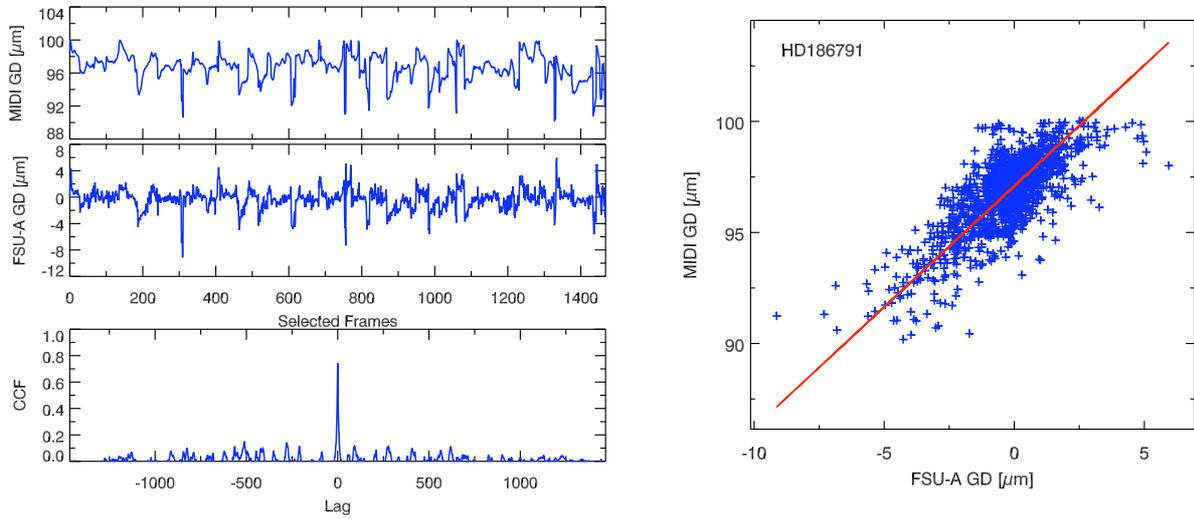
Figure 2. Upper left: MIDI group delay of selected “good” frames and the  $K$  band group delay measured by FSU-A displayed in the middle left plot. Lower left: cross correlation function between both group delay values. Right plot: MIDI group delay vs. FSU-A group delay. The red line is a linear fit with slope one.
