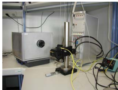
Figure 5 Test bench for testing of the bare mux within a point light source, including IRACE front-end electronic
