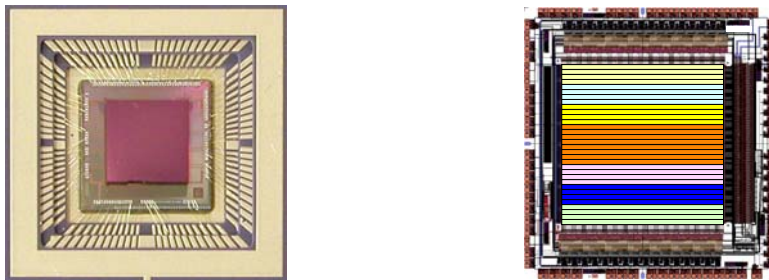
Figure 1 on the left the CALICO IR device, on the right the conceptual die floor-plan showing 7 different pixel designs.
