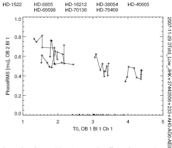
Figure 9. The seeing conditions of the night of 2007, Nov 29, varied sufficiently enough to reveal a correlation between the FINITO performance (as expressed by the phase RMS), and the coherence time  $t_0$  (in this case just Fried's parameter  $r_0$  divided by the wind speed, measured by the ambient seeing monitor on Paranal). The data corresponding to the two P2VM calibrations of this night have been combined for this plot.
