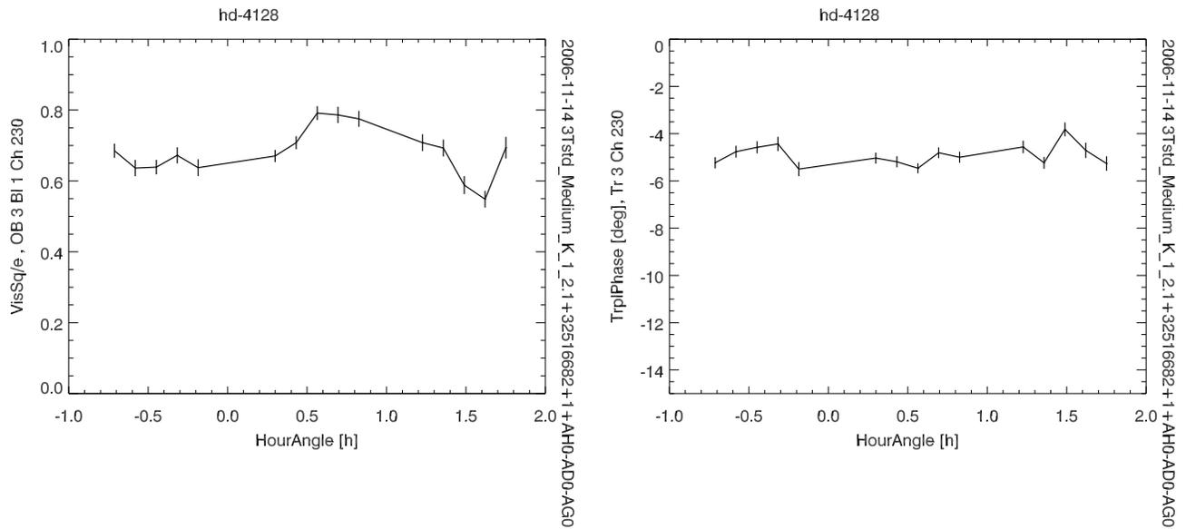
Figure 4. The K-band TF of medium resolution (MR) observations is shown. The MR TF tends to be higher than the LR TF, and the closure phases are much more stable. The measured closure phase offset is relative to the PVM defined zero point, and is used to correct the closure phases of the science targets to which the same P2VM applies.
