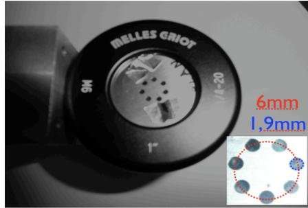
FIG. 8. Mechanical support of the mini-lenses.
