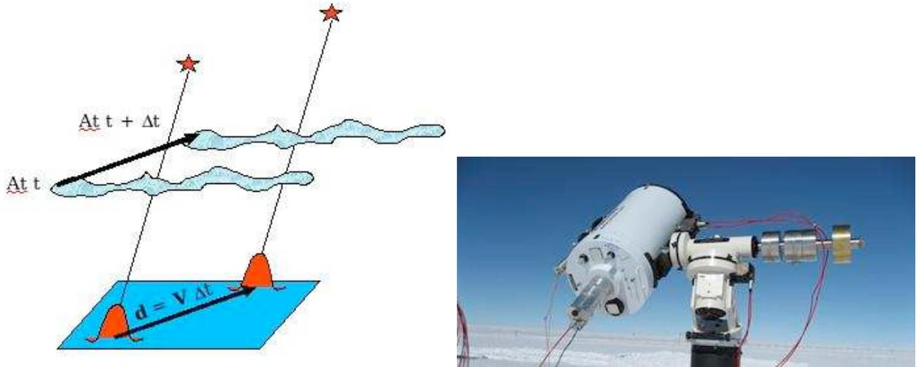
Figure 8. Left: SSS principle. Right: SSS prototype in operation at Dome C. The same instrument is installed at “Observatoire de la Côte d’Azur” in the framework of ELT-DS .
