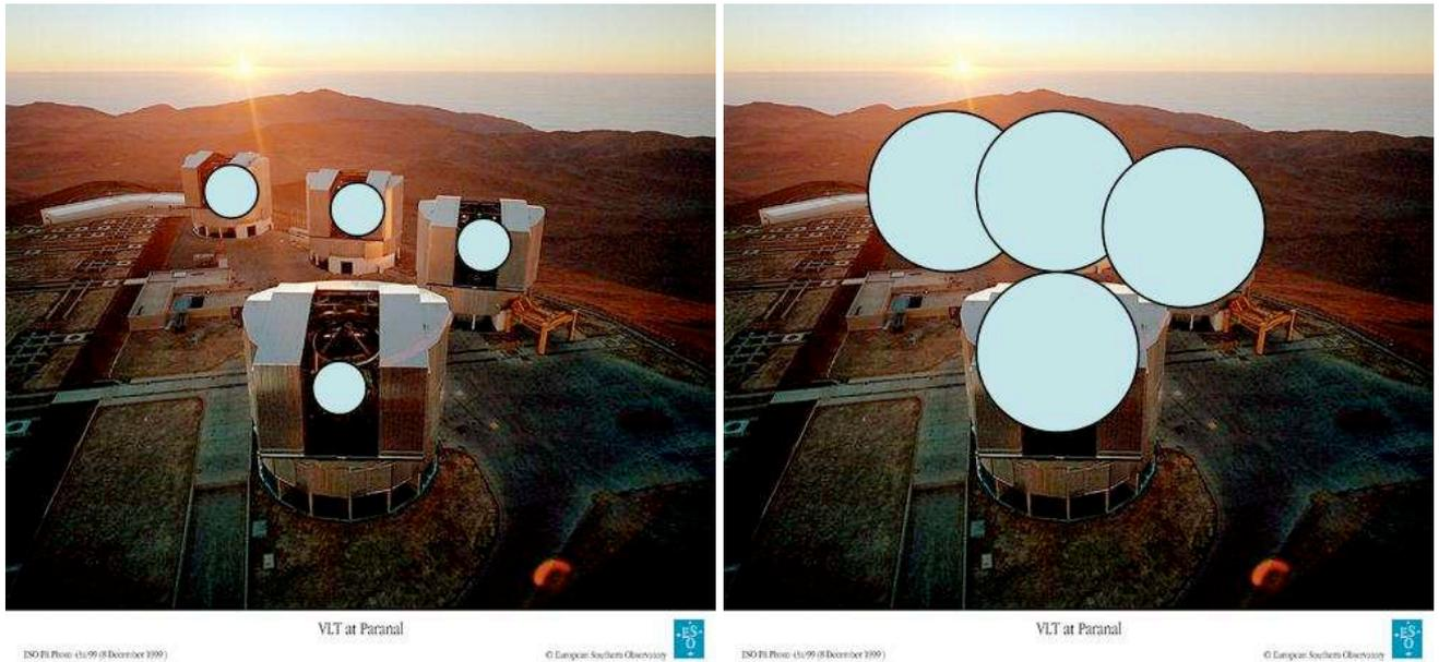
Figure 10. Left: Seen from a single star, one can probe four 8 m wave front. Right: Seen from many stars within a 8 arcmin field of view, at 45 degrees from zenith and for a layer moving at 10 km altitude, one can notice that each pupil is larger and they begin to overlap, allowing a full reconstruction of the wavefront over  $\sim 100$  m.
