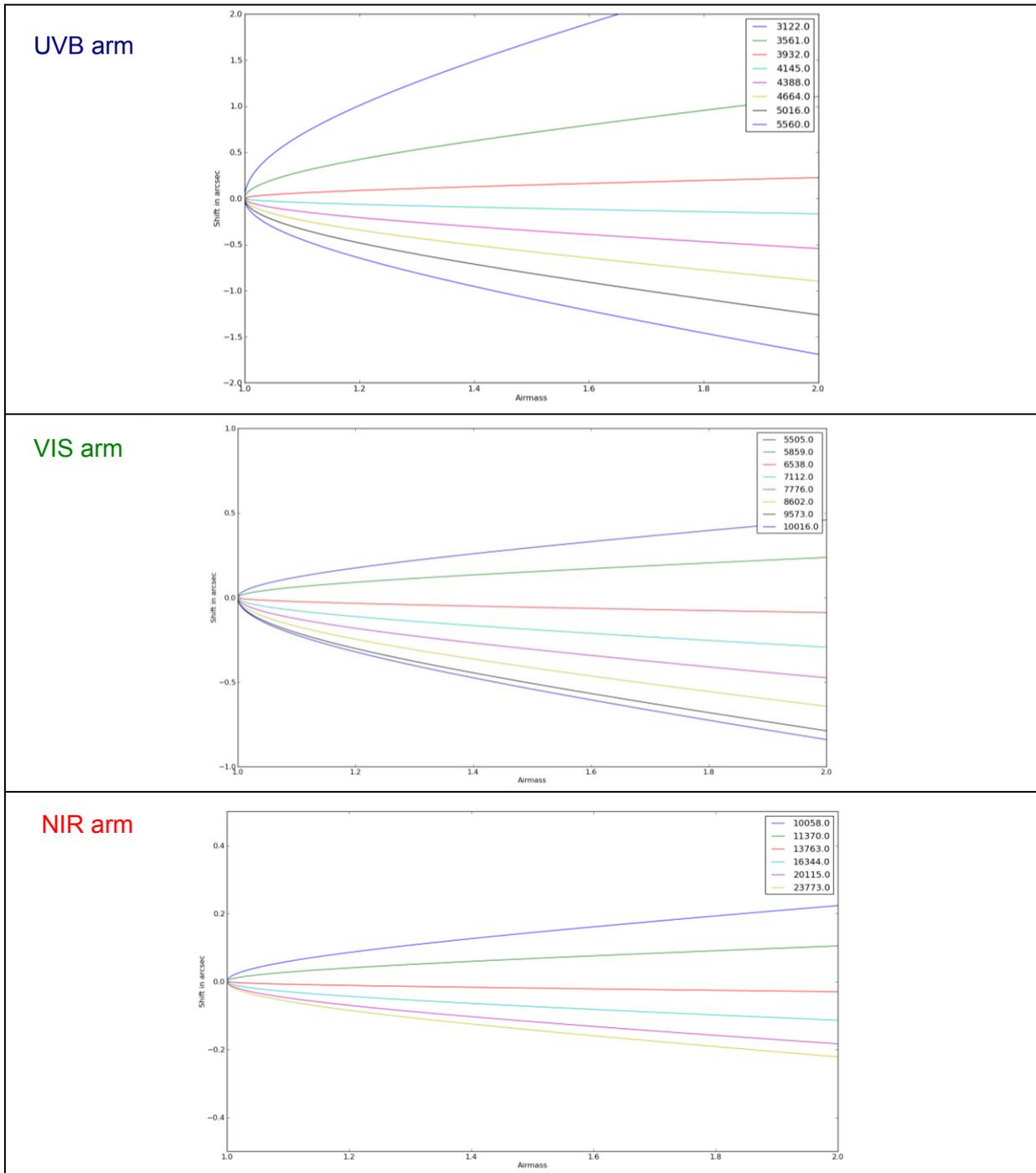
Atmospheric dispersion effect (no ADCs) on the position of the spectrum inside different orders depending on the airmass and the arm (UVB:top, VIS: middle, NIR:bottom). The wavelength is in Angstroms.
