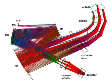
Figure 8: The NIR spectrograph optical layout.
