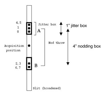
Figure 17: conventions used for nodding of 4" along slit observations. The sequence illustrated here corresponds to 4 cycles (8 exposures, ABBAABBA) with a jitter box of 1".
