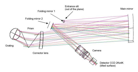
Figure 7: The UVB spectrograph optical layout
