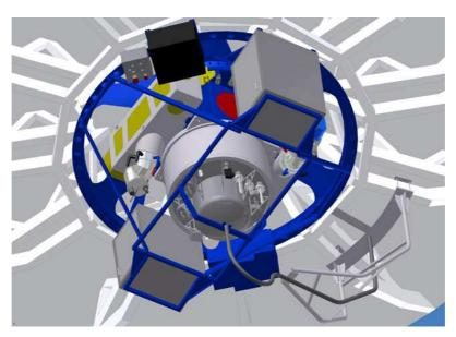
Figure 1: 3D CAD view of the X-shooter spectrograph at the Cassegrain focus of one of the VLT Unit Telescopes.
