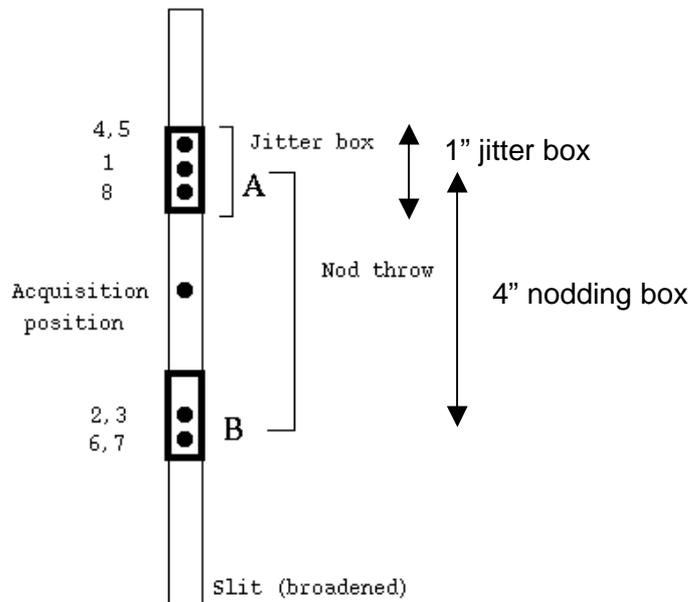
Figure 17: conventions used for nodding of 4" along slit observations. The sequence illustrated here corresponds to 4 cycles (8 exposures, ABBAABBA) with a jitter box of 1".
