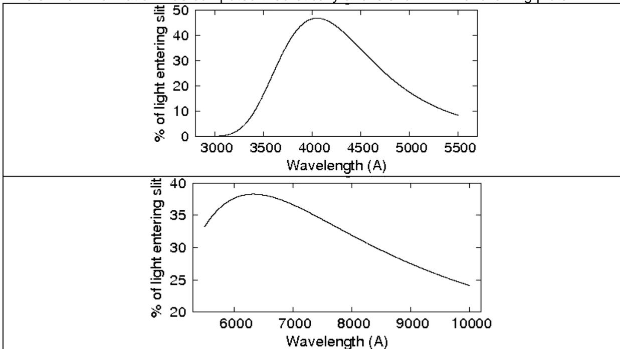
On those plots for observations at 90 degrees of the parallactic angle, slits of 0.4" in the UVB arm (top), 0.5" in the VIS arm (bottom) and a seeing of 0.8" have been considered.
