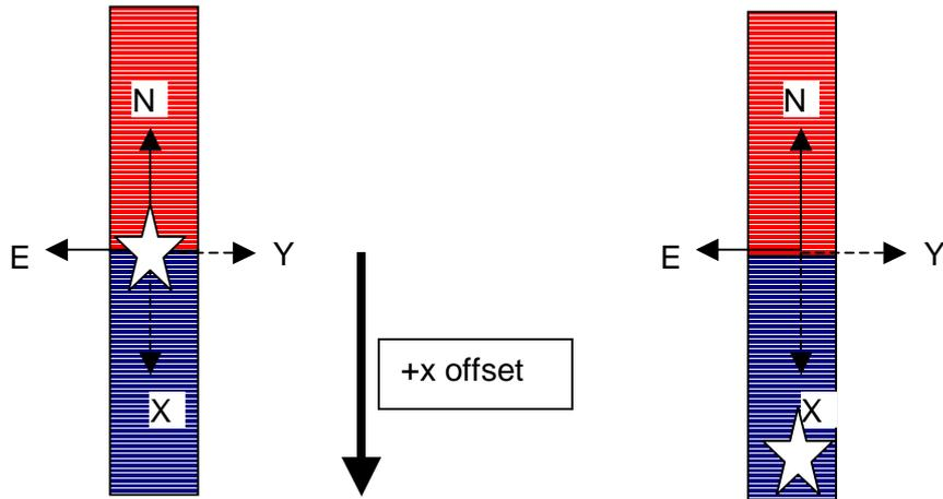
**The second offset with PA= +45 degrees shows a positive offset in y axis.** The Moon goes to the upper right corner (movement in +y axis), while the slit moves in the lower left corner (reverse movement in the -y axis).
