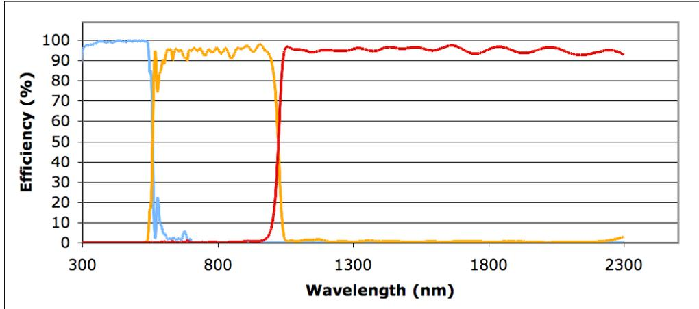
Figure 6: The combined efficiency of the two dichroic beam splitters. *In blue*: reflection on dichroic 1; *in orange*: transmission through dichroic 1 and reflection on dichroic 2; *in red*: transmission through dichroics 1 & 2.
