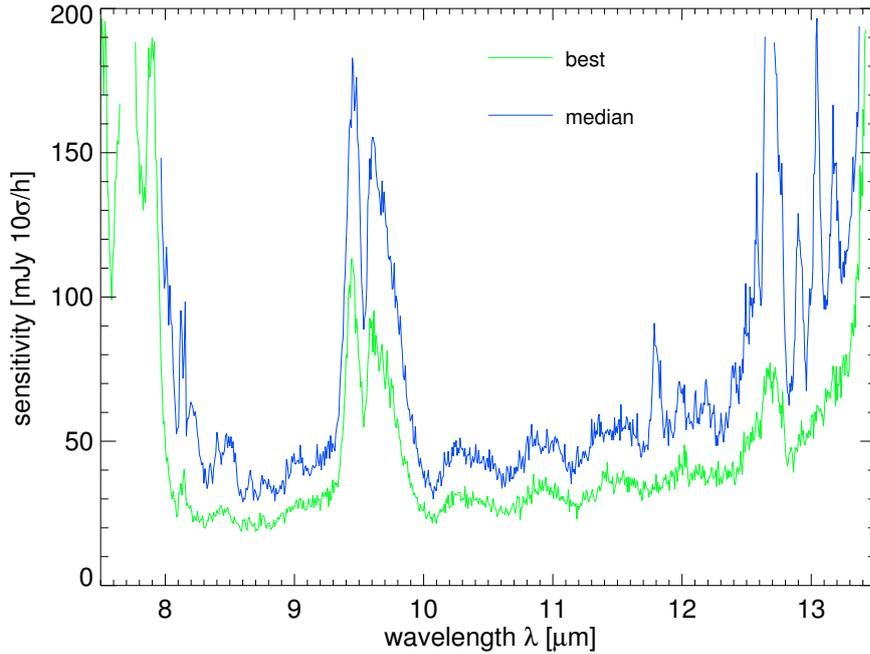
Figure 10: Median and best low resolution sensitivities [mJy/10 $\sigma$ /h] observed during comissioning 2 under mediocre atmospheric conditions.
