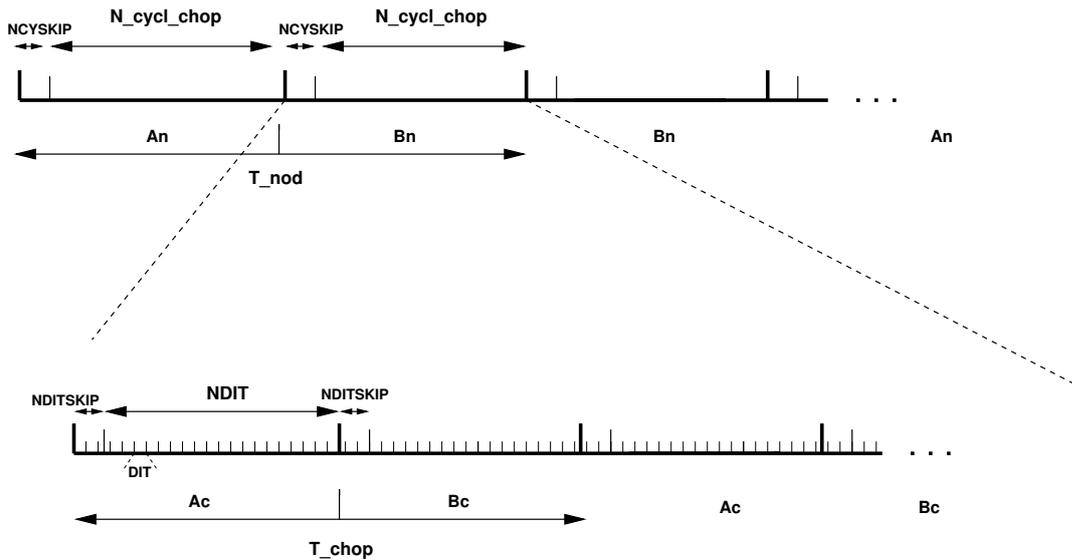
Figure 15: Data timing in VISIR.  $A_c$  and  $B_c$  refer to the two chopper positions,  $A_n$  and  $B_n$  refer to the two nodding (telescope) positions. Note the  $A_n B_n B_n A_n$  cycle sequence for the nodding to save observing time.
