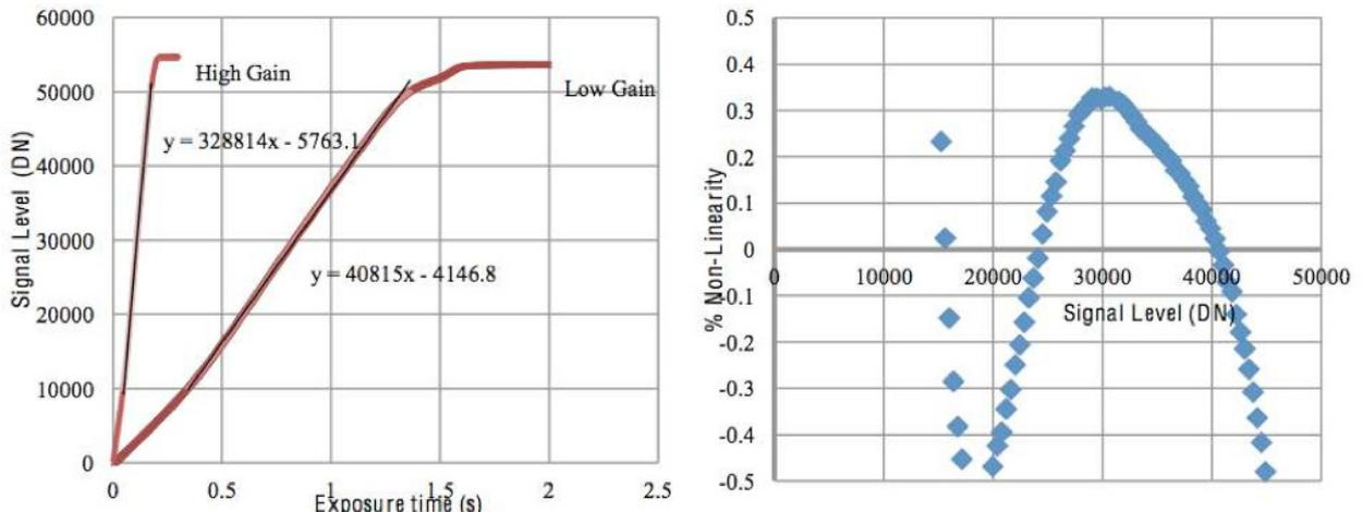
Figure 13: Left panel displays the measured AQUARIUS detector linearity for both high and low gain read modes. Right panel displays the non-linearity as a function of the signal level, as computed for the high gain setup.
