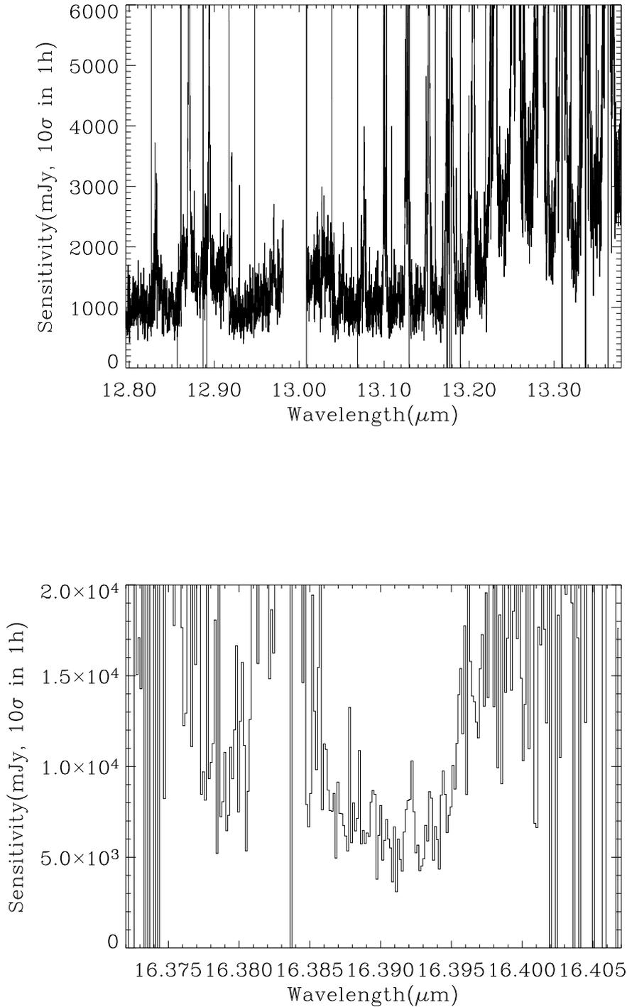
Figure 23: Observed sensitivity measured for the old DRS detector as a function of wavelength for high resolution mode (IV). Offered sensitivity is typically a factor of 2 larger and still valid until new measurements are available. *Top*: Sensitivities over an extended region encompassing the observed wavelength of [NeII] up to  $z \approx 0.038$ .
