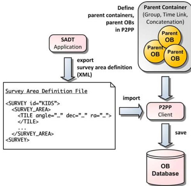
Figure 12. Definition of a Survey Area using SADT and import into P2PP
