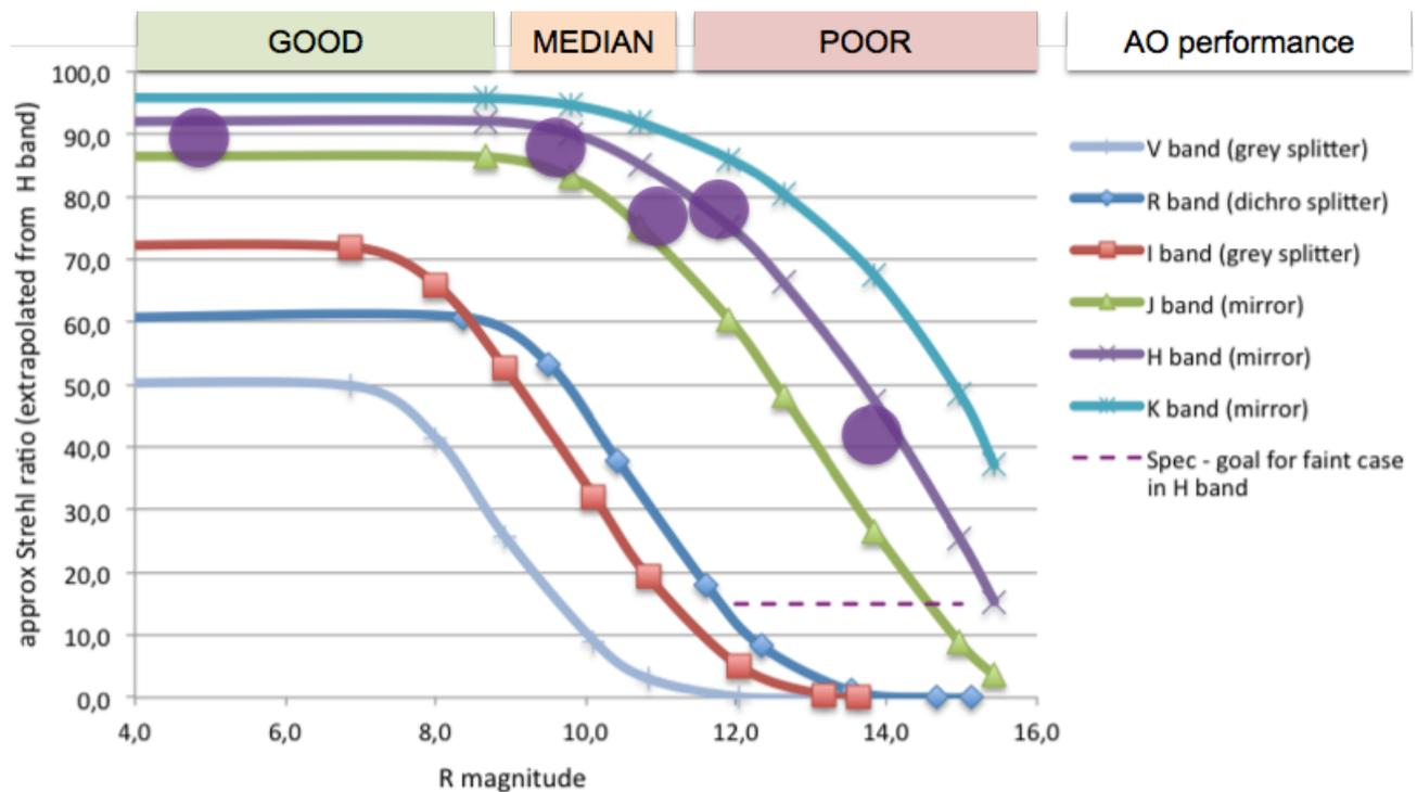
Figure 10: Theoretical and measured (purple circles) SPHERE-SAXO Strehl ratio as a function of R magnitude for good seeing conditions and different wavelength ranges from V to K (see Table 9 and Table 10 for details).
