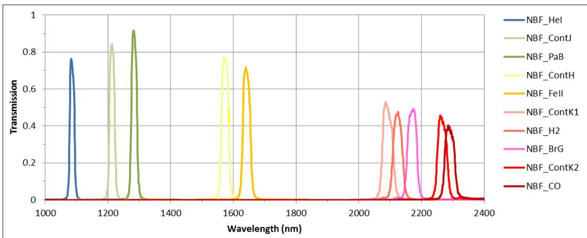
Figure 31: IRDIS NB filters.
