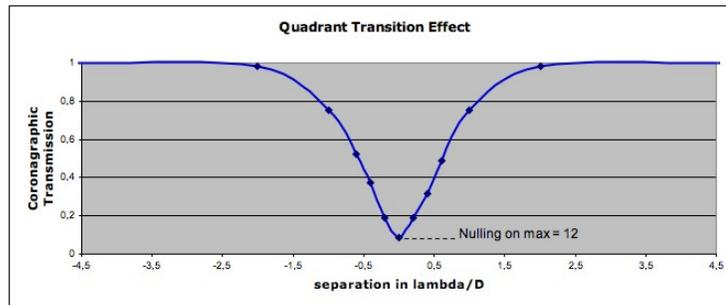
Figure 31: Relative transmission curve of the 4QPM across a phase transition between two adjacent quadrants.
