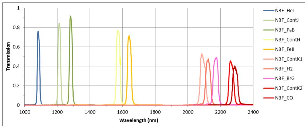
Figure 29: IRDIS NB filters.
