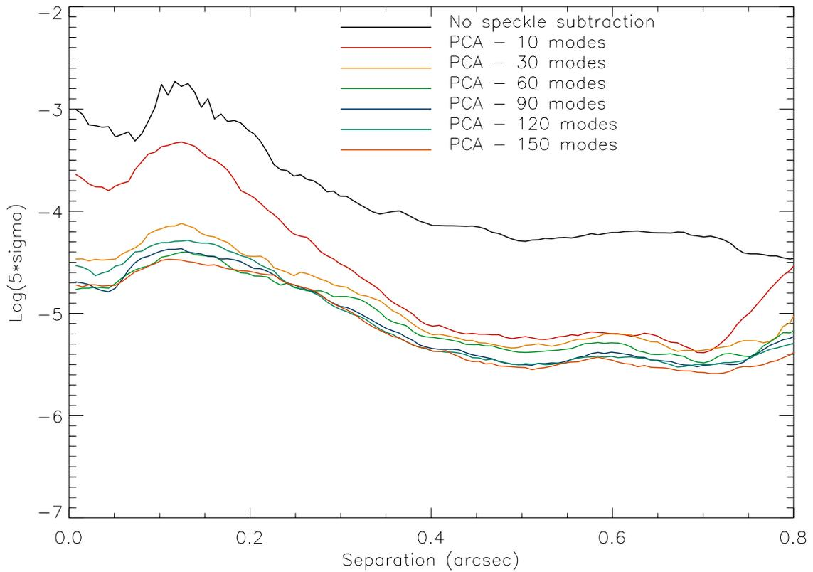
Figure 18: IFS  $5\sigma$  sensitivity on Iota Sgr as function of angular separation, for different principal components retained in the speckle subtraction using both spectral and temporal diversity (ADI).
