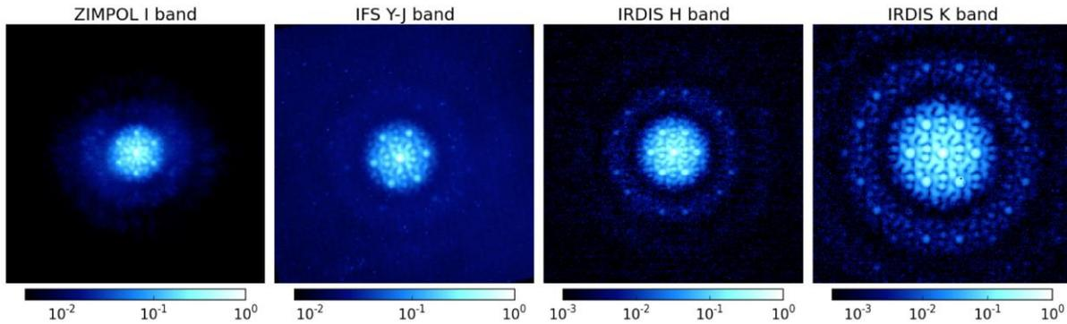
Figure 23: SAM\_7H on-sky point spread functions for 4 observing wavelengths with 3 cameras: a ZIMPOL I band exposure, a IFS wavelength slice between Y and J bands, an IRDIS H band image and an IRDIS Ks band image.
