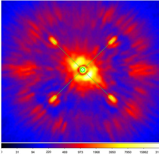
Figure 44. Irdis image in broad-band H, with the N\_ALC\_YJH coronagraph, with the waffle pattern applied to the DM, creating four satellite spots. These spots are elongated with broad-band filters and point source with narrow-band filters. The green lines start and end points were computed by fitting a 2D Gaussian on each spot, they intersect on the star center, indicated by a green thick circle.
