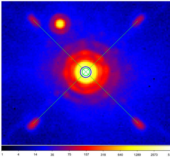
Figure 45 Non coronagraphic image of a star (happening to have a binary companion) in broad-band H with Irdis, after applying a waffle pattern to the DM for calibration purposes. The green thick circle indicates the intersection of the green lines, while the blue thick circle indicates the star position (Gaussian fit). Both agree within 2.5mas.
