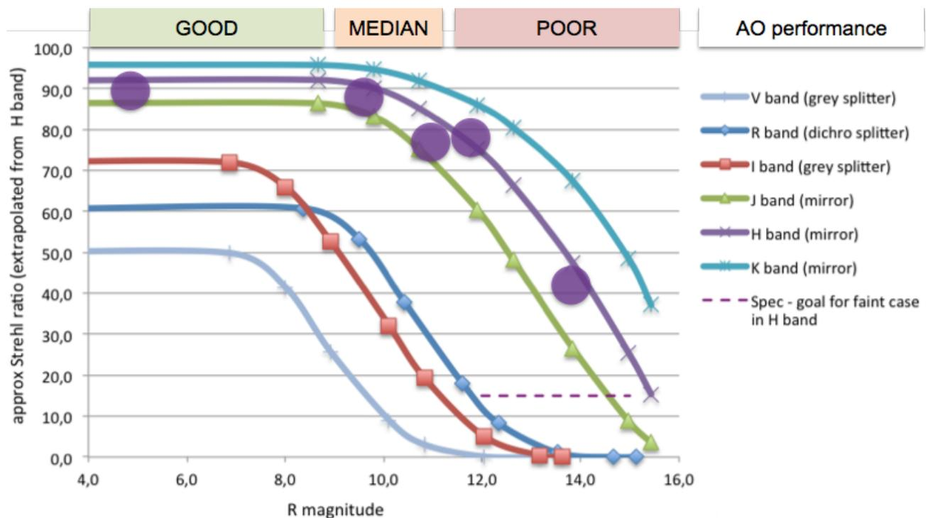
Figure 11: Theoretical and measured (purple circles) SPHERE-SAXO Strehl ratio as a function of R magnitude for good seeing conditions and different wavelength ranges from V to K (see Table 10 and Table 11 for details).
