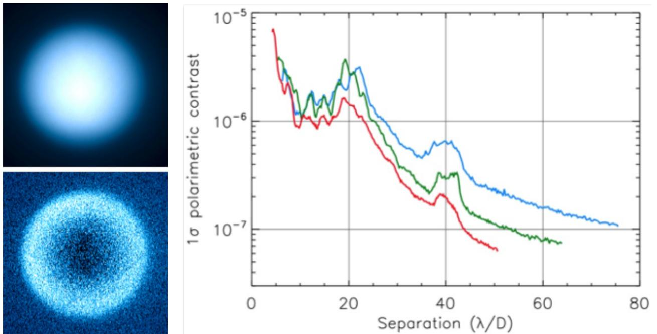
Figure 22: Top left: intensity image of Titan. Bottom Left: polarized intensity. Right: polarimetric contrast (right) on a bright target for the V (blue), N\_R (green), N\_I (red) filters.
