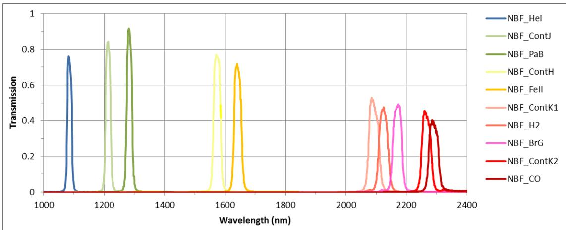
Figure 39: IRDIS NB filters.
