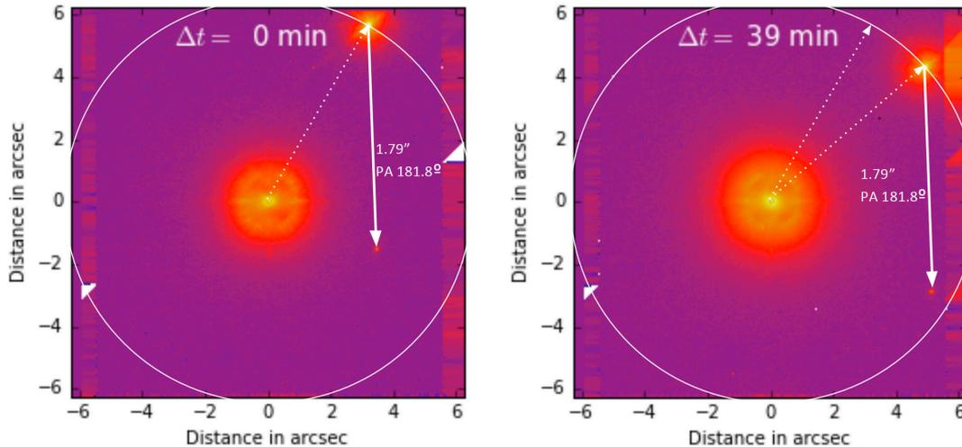
Figure 36: IRDIS ghost appears when there is a bright source on upper right corner of detector.
