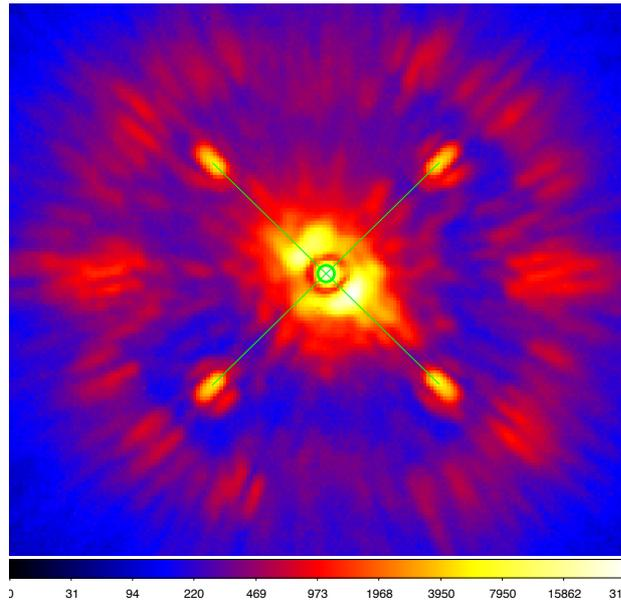
Figure 42. Irdis image in broad-band H, with the N\_ALC\_YJH coronagraph, with the waffle pattern applied to the DM, creating four satellite spots. These spots are elongated with broad-band filters and point source with narrow-band filters. The green lines start and end points were computed by fitting a 2D Gaussian on each spot, they intersect on the star center, indicated by a green thick circle.
