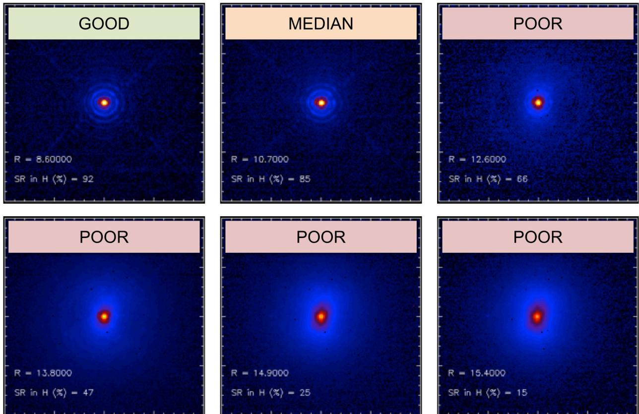
Figure 12: SPHERE PSF morphology and Strehl ratio as a function of R magnitude (see Table 10 and Table 11 for details).
