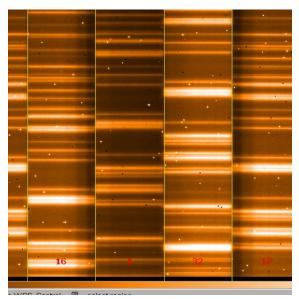
Fig. 3: Sky spectra showing the vignetting of slit#32 (labelled at the bottom) is much reduced. There is still significant vignetting in slit#1 (note however that the "blind spot" also lies partially on this slit).
