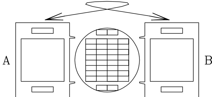
Figure 12: Orientation of a filter depends on whether it is loaded in magazine A or B.
