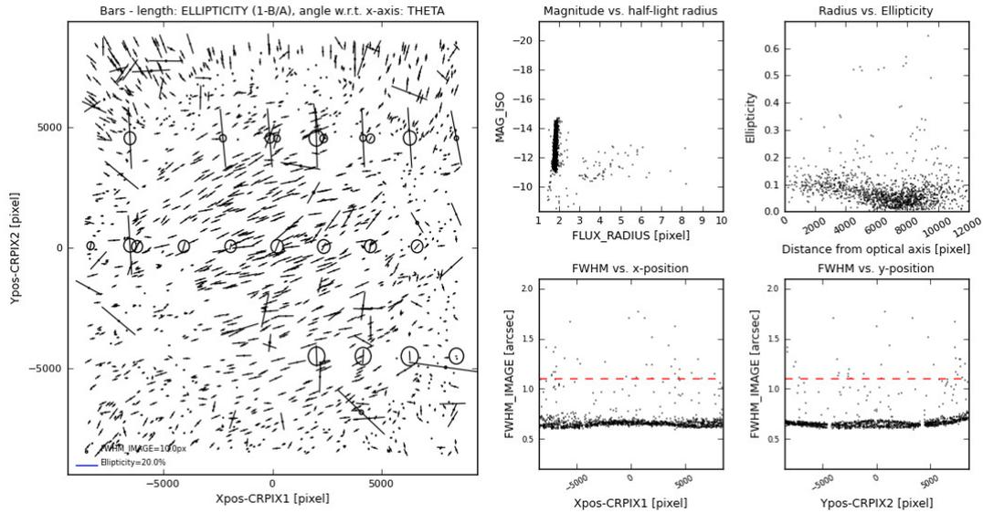
Figure 24: PSF anisotropy analysis plot obtained for an i-band observation. For the given example, outside seeing as indicated by the DIMM (around V-band) was  $0.9''$ , and IQ on OmegaCAM chips was  $\sim 0.65''$ . In general, IQ variations of 10-25% across the FOV can occur, depending on outside seeing, filter and telescope mirror position.
