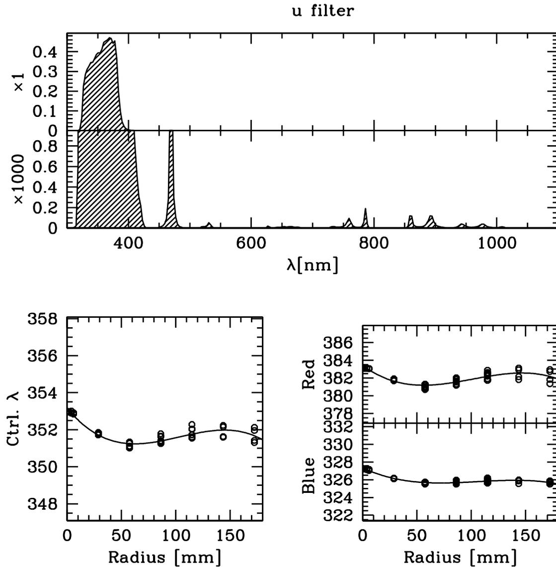
Figure 34: Top panels: throughput of the  $u'$  filter  $\times$  average CCD response curve, including a blow-up by a factor of 1000 to show the out-of-band blocking. Bottom left: variation of central wavelength with radius on the focal plane (dots: measurements; line: polynomial fit). Bottom right: corresponding variation of wavelength at half-maximum throughput of the blue and red edges of the filters. The edge of the CCD array is reached at a radius of  $\sim 180$ mm.
