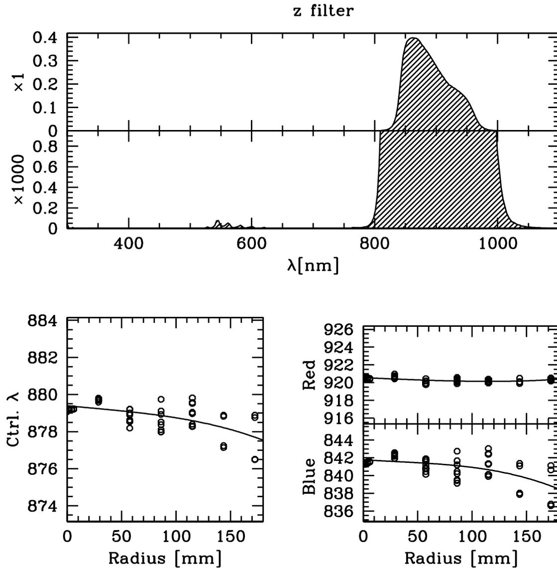
Figure 38: Top panels: throughput of the  $z'$  filter  $\times$  average CCD response curve, including a blow-up by a factor of 1000 to show the out-of-band blocking. Bottom left: variation of central wavelength with radius on the focal plane (dots: measurements; line: polynomial fit). Bottom right: corresponding variation of wavelength at half-maximum throughput of the blue and red edges of the filters.
