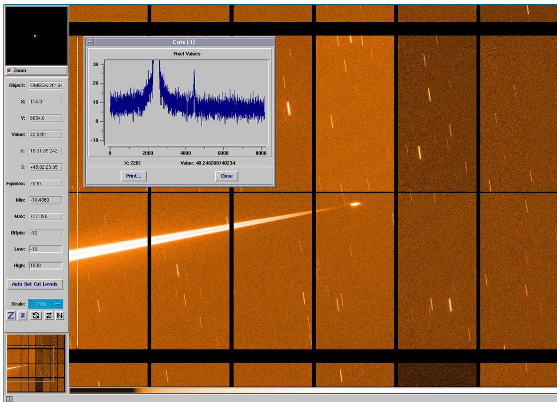
Figure 19: Reduced observations taken in clear conditions with no Moon of the in-focus 4LGSF laser with OmegaCAM in r\_SDSS with 20s of exposure time without tracking.
