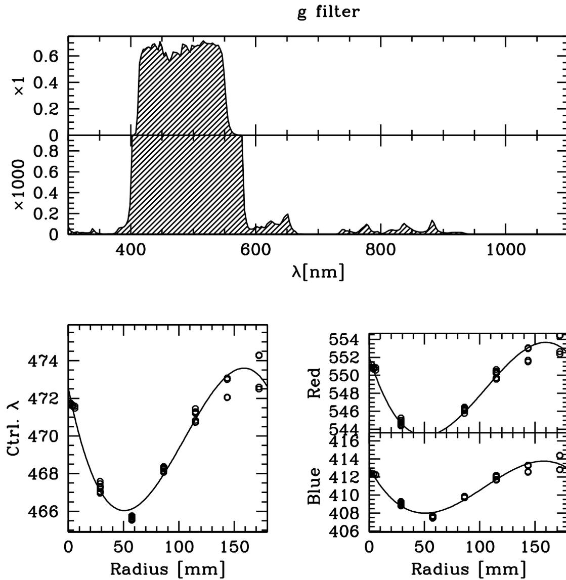
Figure 35: Top panels: throughput of the  $g'$  filter  $\times$  average CCD response curve, including a blow-up by a factor of 1000 to show the out-of-band blocking. Bottom left: variation of central wavelength with radius on the focal plane (dots: measurements; line: polynomial fit). Bottom right: corresponding variation of wavelength at half-maximum throughput of the blue and red edges of the filters.
