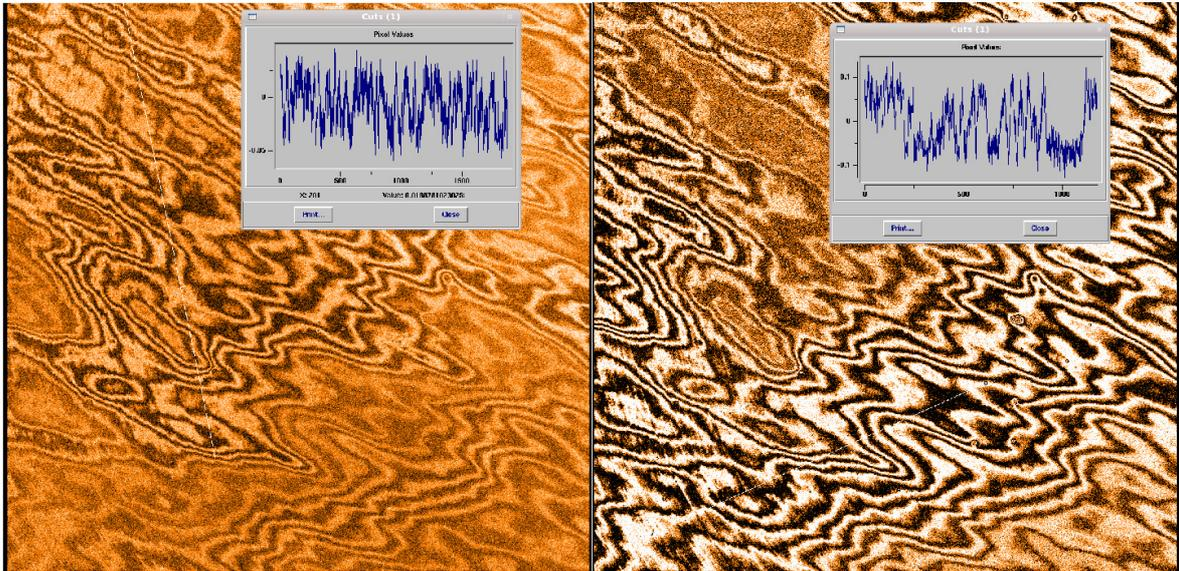
Figure 30: excerpts of a fringe map for the Sloan  $i'$  (left) and  $z'$  band (right). Intensity contrasts in the image are at  $\pm 5\%$ . The cuts show that fringe amplitudes are a few percent in  $i'$ , and up to 10% in  $z'$ .
