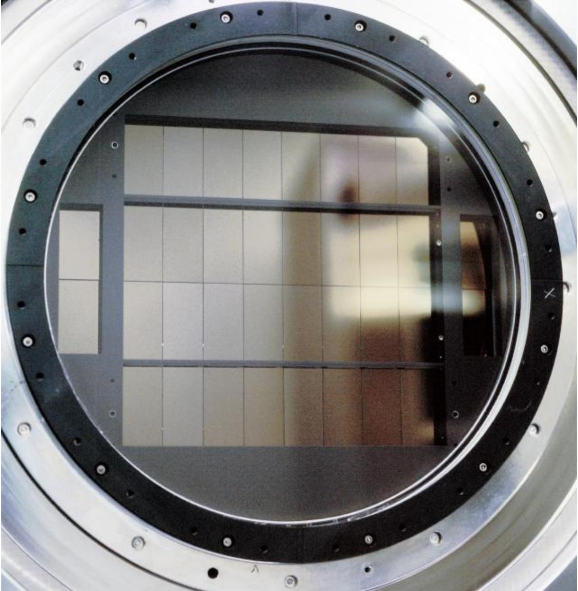
Figure 5: Picture of the 36 CCDs mounted behind the dewar window. Note the black strips that cover the gaps between the CCDs: they prevent reflection of light off the bright bond wires of each detector. Slight vignetting is observed near these strips, and on the long outer sides of the four corner CCDs.
