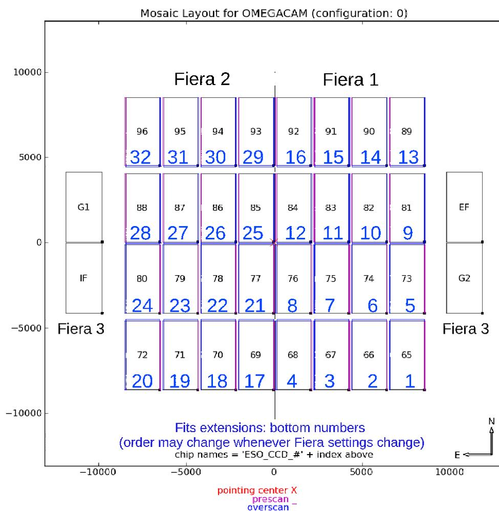
Figure 3: The layout of the 32 science CCDs and the four auxiliary CCDs in the focal plane. The science array covers a 1 degree x 1 degree area of sky, with 16k x 16k pixels of 0.21 arcsec. All CCDs fit inside a circle of diameter 1.4 degrees on the sky. (Note that this is the layout as seen from below, i.e., the projection of the array onto the sky.)
