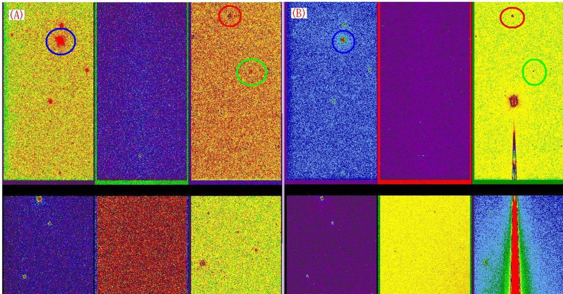
Figure 22: (A) A 300s exposure taken with the NB659 filter and OmegaCAM (B) A 20s exposure taken using the r\_SDSS filter on the same field. In both cases the PARLA laser was propagating (somewhat less powerful than the new 4LGSF system). Blue, red and green circles show stars visible on both images. The images are raw (no reduction has been performed). No laser light is visible when using the NB659 filter.
