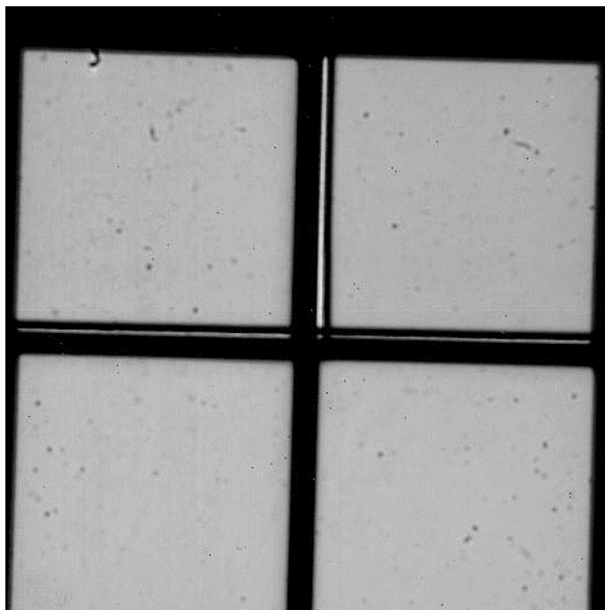
Figure 4-8: Flat field image of the SDI+ mode. The transmitted wavelengths are 1.6 mm (top left), 1.575 mm (top right) and 1.625 mm (bottom left and right).
