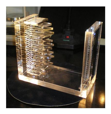
**Figure 6:** MUSE Field splitter and field separator optics. The 24 mirrors positioned at varying angles split the MUSE field-of-view in 24 horizontal bands.
