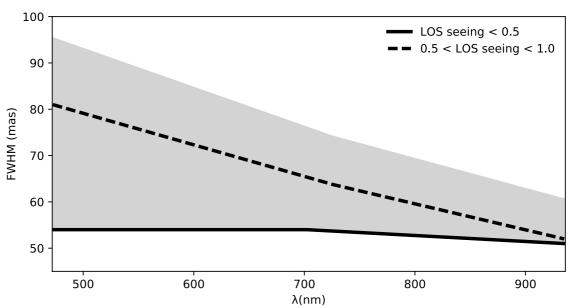
**Figure 23:** FWHM of the MUSE NFM PSF peak as a function of wavelength. The solid line represents the very best performance in the best seeing conditions with a seeing (at 500 nm) along the line of sight (LOS) <0.5". The dashed line shows the median performance for a seeing along the line of sight between 0.5" and 1.0". The grey area shows the observed variation of the FWHM recorded during the commissioning runs, depending on details of the atmospheric turbulence profile.
