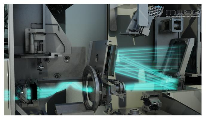
Figure 4: Drawing of rays in the fore-optics, from the de-rotator to FOWMtM1.
