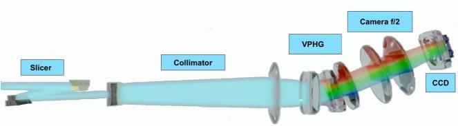
**Figure 8:** Overview of the optical layout for one of the IFUs. The top panel shows one of the slicers, which cuts the FOV of each channel into 4 stacks of 12 slices. The bottom panel shows the optical elements in the IFU and the path of light to the CCD.
