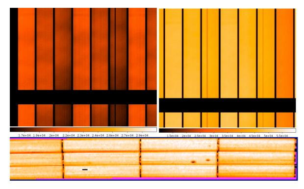
**Figure 21:** Dark features in the MUSE flat fields due to dust in the field splitter. Top: the regions of low transmission extend the full length of the spectrum. On the left is an N-mode flat and on the right is an E-mode flat. Bottom: the 'spots' of low transmission in a reconstructed datacube.
