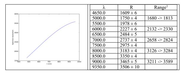
**Figure 17:** Spectral resolution,  $R = \lambda/\Delta\lambda$ , as a function of wavelength, as measured in the lab using calibration lamps. <sup>1</sup>Range over channels. From Technical Note ESO-318117.
