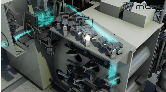
**Figure 7:** 3D view of optical paths for all channels due to the relay optics splitting of the field-of-view into 24 channels. The bottom figure shows the path of light rays for one of the channels, as seen from the Fore-Optics.
