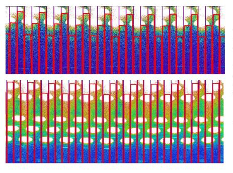
Figure 19: Second order effect in nominal (top panel) and extended (bottom panel) modes, here for a bright exposure with arc lines. The red boxes mark the slice limits up to 930 nm. The impact of second order is visible as the white ellipses illuminating the top of nominal detector. The instrument mode is not affected by contamination, but it is more significant in the extended instrument mode.
