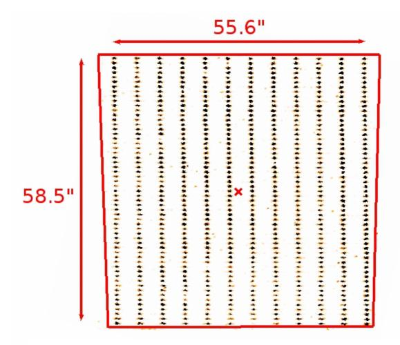
Figure 30 Arrangement of the WFM SMP mask used for geometrical calibration, as viewed on a reconstructed image when illuminated with internal lamps. We overlay the trapezoidal shape of the FOV in red.
