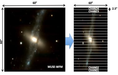
Figure 10: Overview of the splitting of the field-of-view from the fore-optics to one of the MUSE detectors. Left: splitting of the MUSE FOV into 24 sub-fields entering each channel. Center: shape of the entrance slicer on sky, with 4 stacks of 12 slices (numbered in red from 1 to 48) covering a 2.5" x 60" field. Bottom: location of each slice on the detector, with the corresponding wavelength range.
