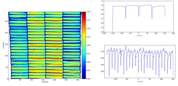
**Figure 18:** (left) normalized reconstructed image of the continuum flat-field in WFM. (right) horizontal (top) and vertical (bottom) cuts through the normalized image showing the horizontal and vertical variations in illumination.
