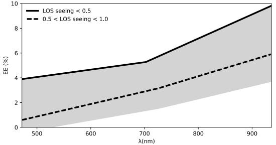
**Figure 24:** Ensquared Energy (EE) in a 25mas (one spaxel) box as a function of wavelength. As in, Figure 23, the continuous line shows the best performance for a LOS seeing <0.5". The dashed line shows the median performance and the grey area indicates the range observed during the commissioning runs for a LOS seeing between 0.5 and 1 arcsec.
