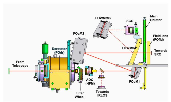
Figure 3 MUSE fore-optics schematics in NFM configuration
