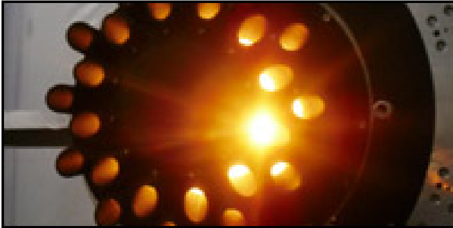
Figure 7: View of the internal calibration unit, showing the 24 output apertures or ports illuminated by the flat-field tungsten lamp.
