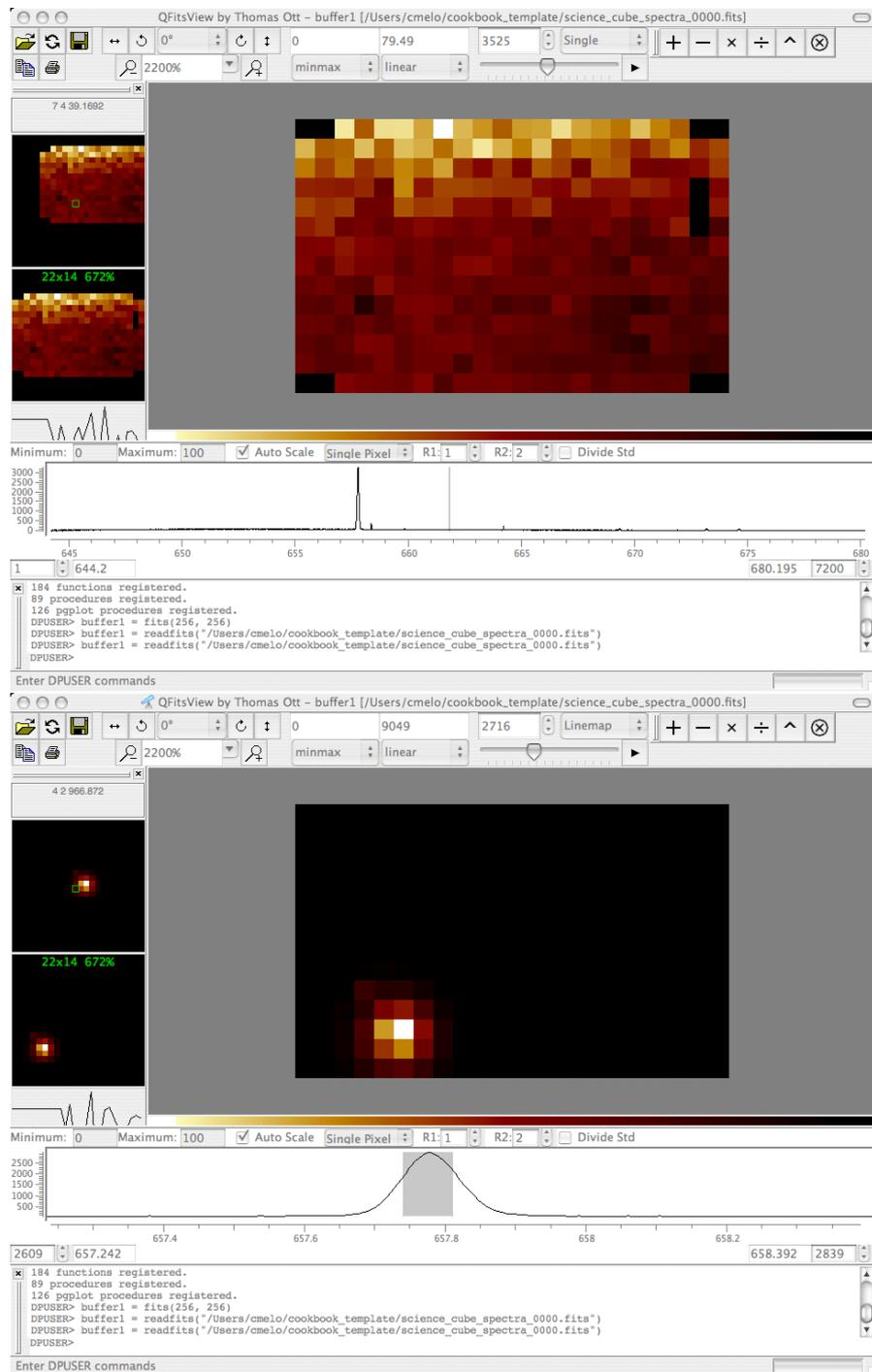
Figure 23: Argus cube of an emission line object produced by the pipeline and visualized by QFitsView. The upper panel show the flat image, i.e, the whole wavelength range is considered. Nothing is really seen with respect to the background. In the lower panel, one the core of the emission is display. The object pops-up with respect to the background.
