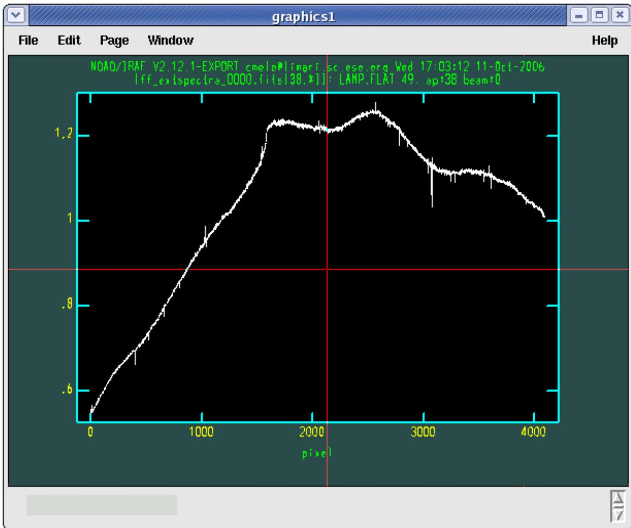
Figure 17: Extracted flat-field spectrum for one the fibers. The spectrum was produced by `gimasterflat` and will be wavelength calibrated by the next step carried out by `giwavecalibration`.
