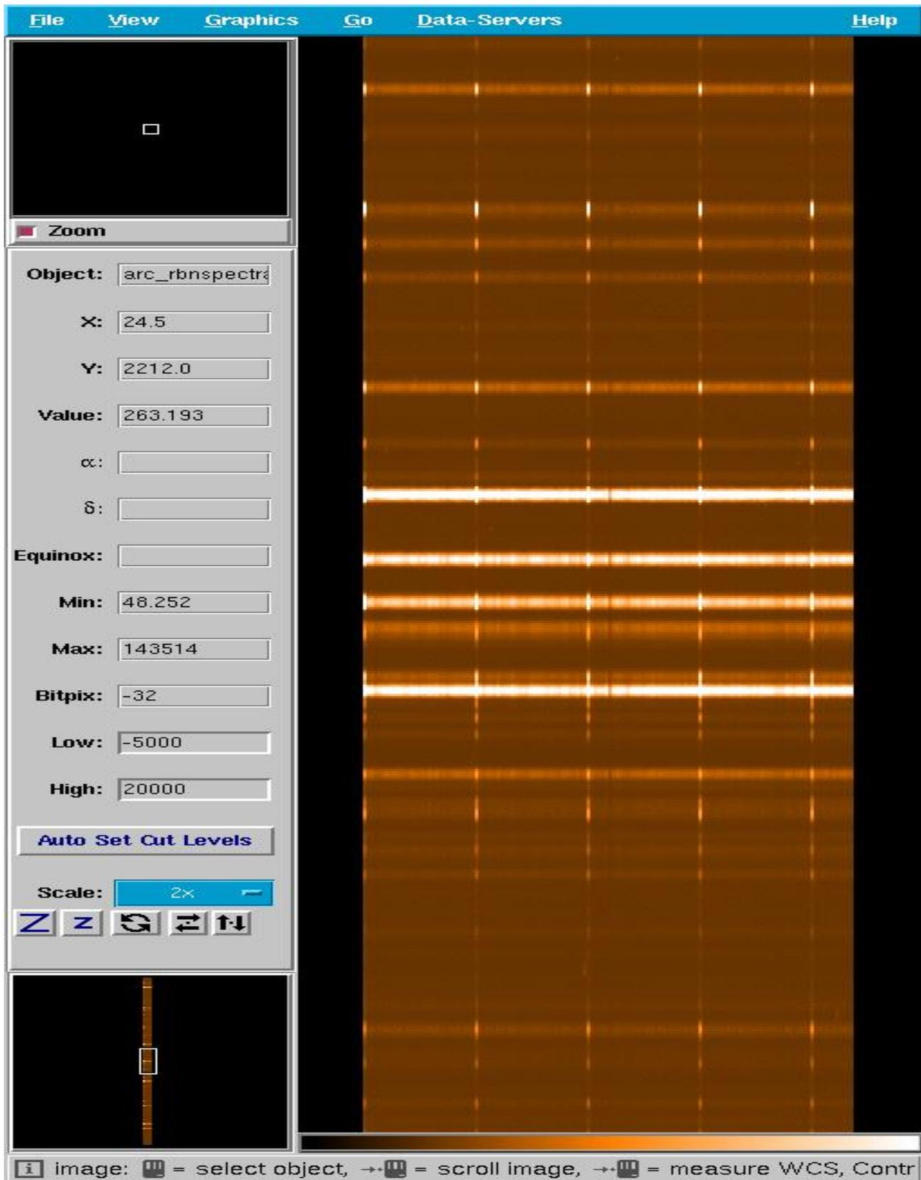
Figure 21: Rebinned arc-line spectrum `arc_rbnspectra.fits` created by `giwavecalibration` after making a new slit geometry table. The jumps in 'y' are much less pronounced than in Fig 19.
