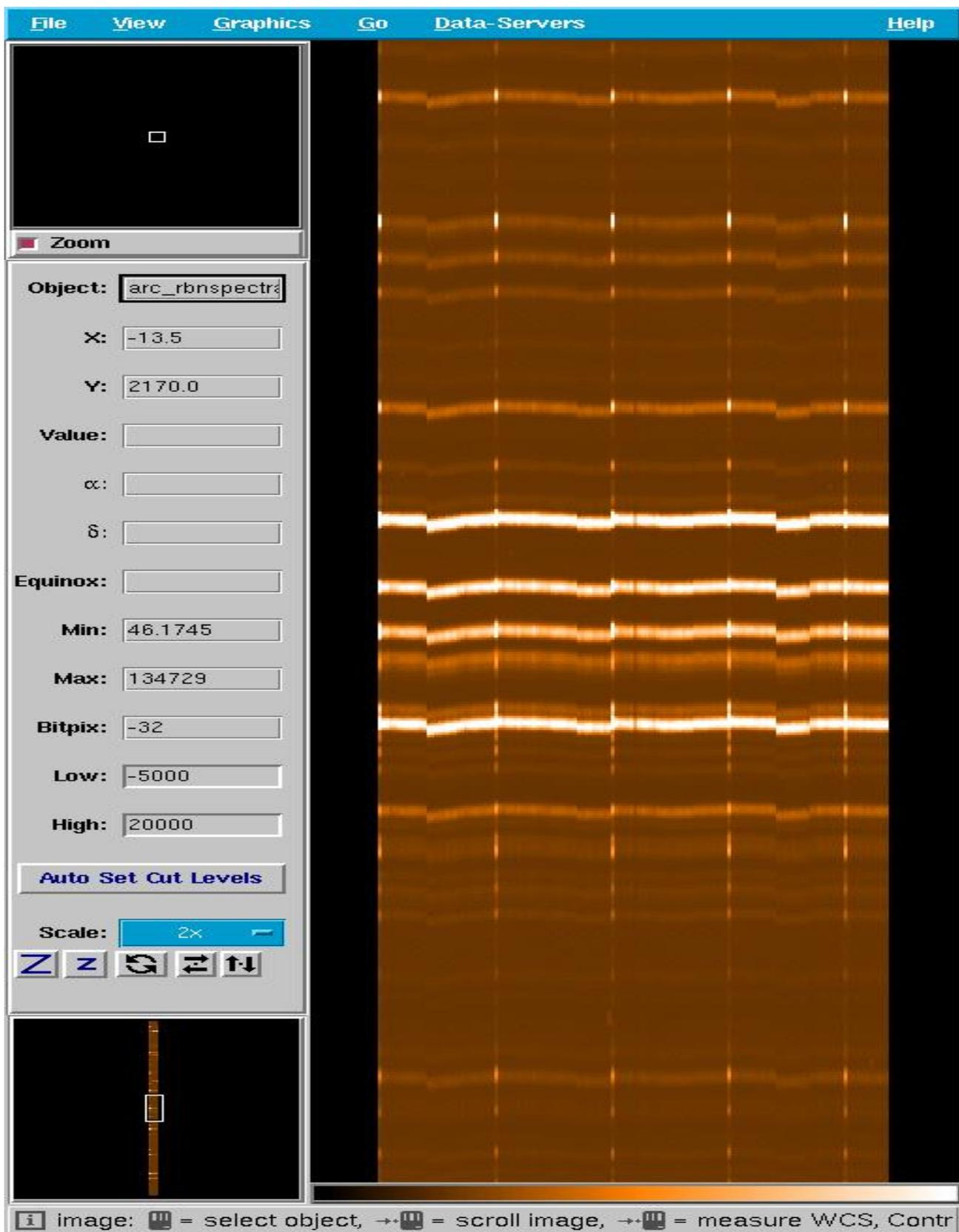
Figure 19: Original rebinned arc-line spectrum `arc_rbnspectra.fits` created by `giwavecalibration`. Jumps in the 'y' position signify that this is not a good wavelength solution and should be improved by creating a new slit geometry table.
