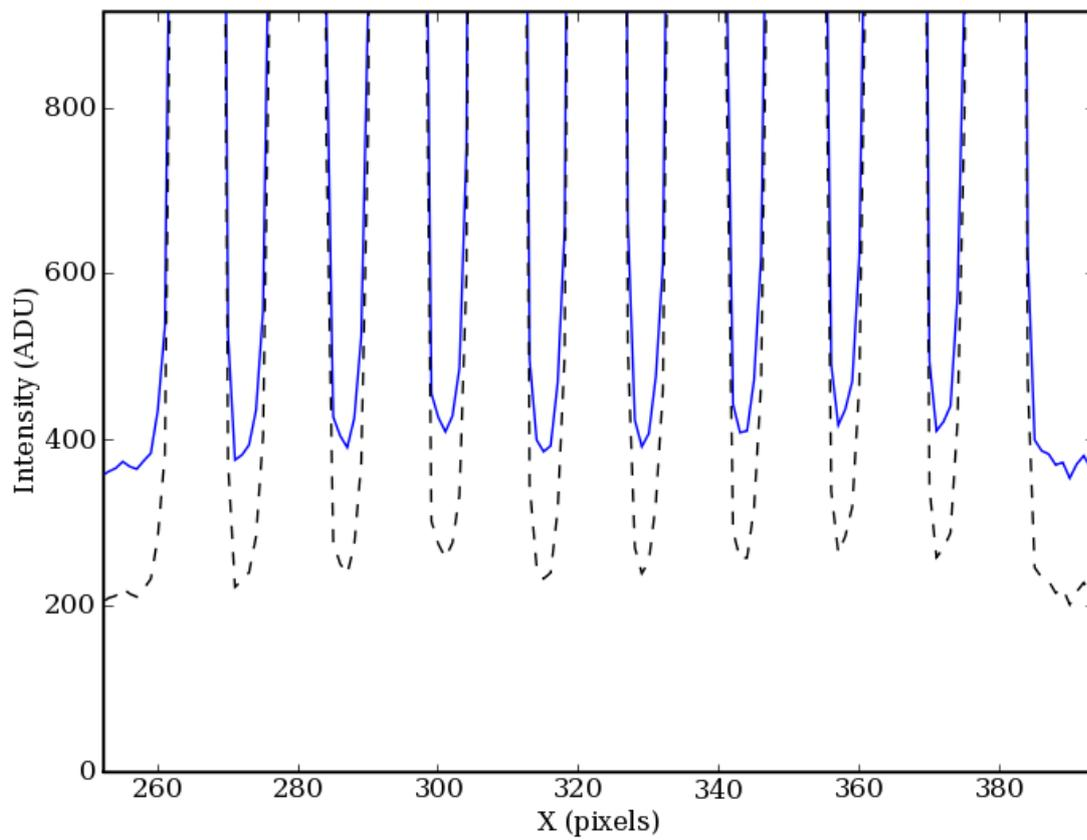
Figure 4: Cut across the fibers. Solid and dashed lines show the minimum level before and after bias subtraction. The remaining ADUs seen in the case of the bias subtracted frame are due to the dark current and scattered light.
