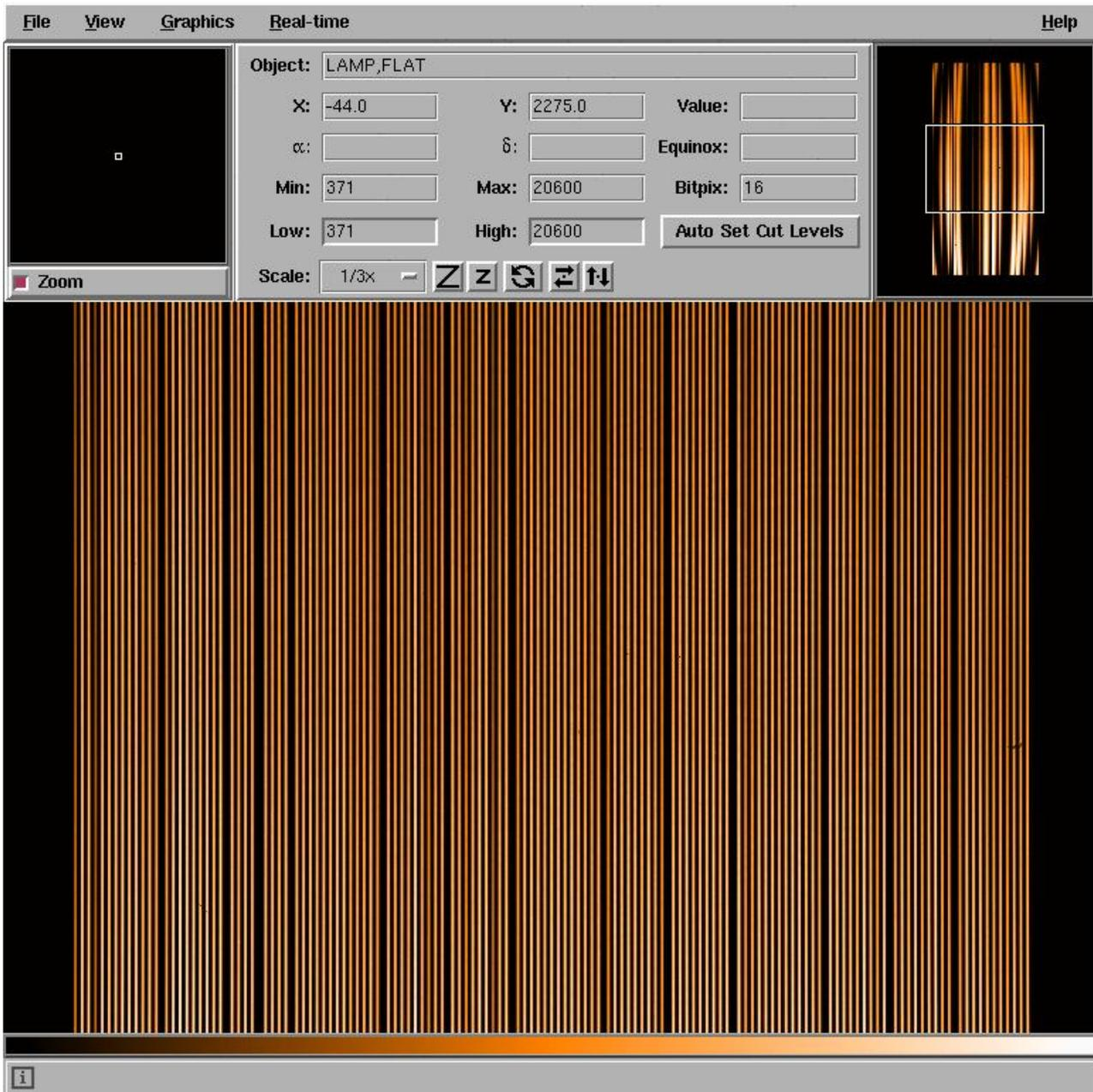
Figure 15: A Medusa1 flatfield image in which fibre 27 (about a quarter from the left) is missing. Note that for ARGUS the counting is done from right to left and not from left to right as in Medusa or IFU.
