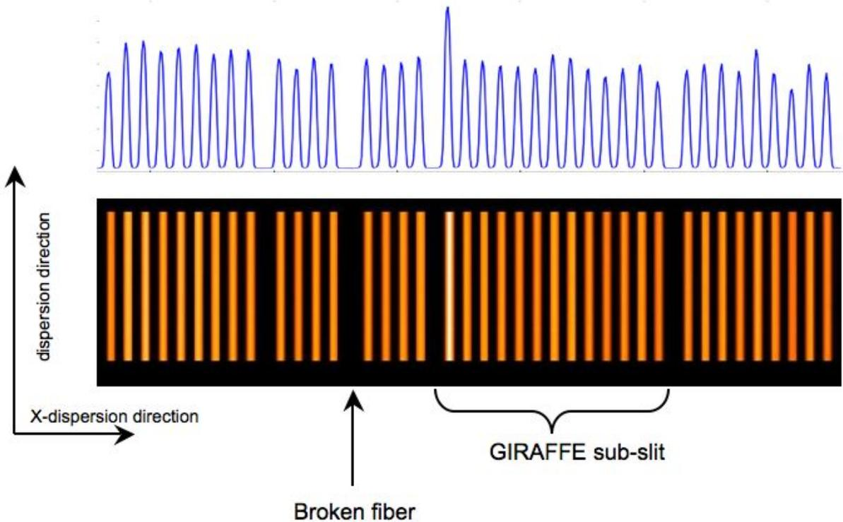
Figure 2: An extract of a raw image of a flat-filed frame is shown the bottom panel. The sub-slits (packets of fibers) defined in the previous figure are clearly seen in the image as well as a broken fiber. In the top panel, a cross section of the frame is shown where the nearly Gaussian profile of the fibers can be seen.
