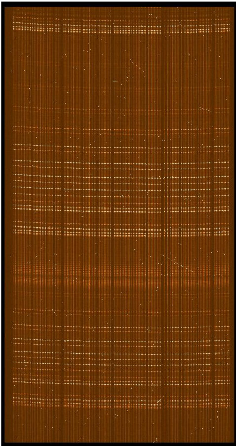
Figure 5: This image shows how especially in the red that there are many sky lines. Removing them can be critical to obtaining good science output. The exposure was taken using GIRAFFE at L881.7-nm for 2750-s.
