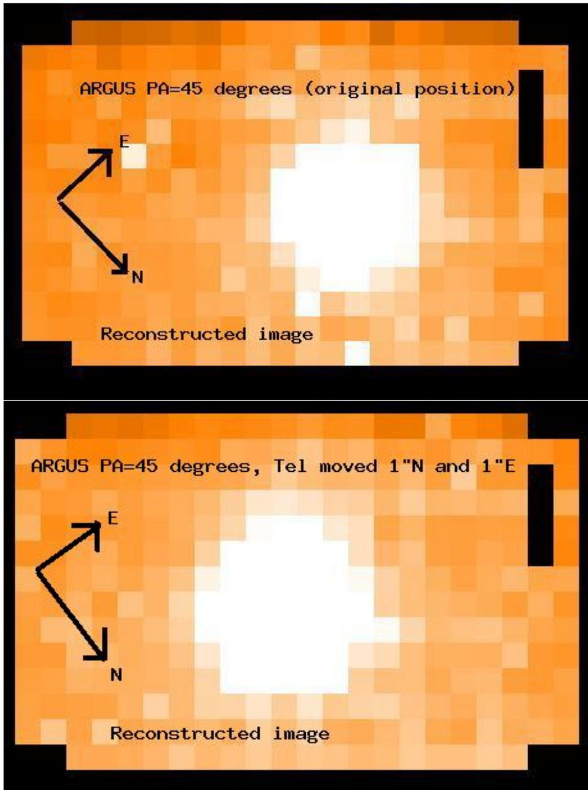
Figure 27: Argus reconstructed image with Position angle in the acquisition set to +45 degrees. Top panel: Original pointing. Bottom panel: Telescope moved by 1.0 arcseconds North and 1.0 arcseconds East i.e. the object moves 1.0 arcseconds South and 1.0 arcseconds West on ARGUS.
