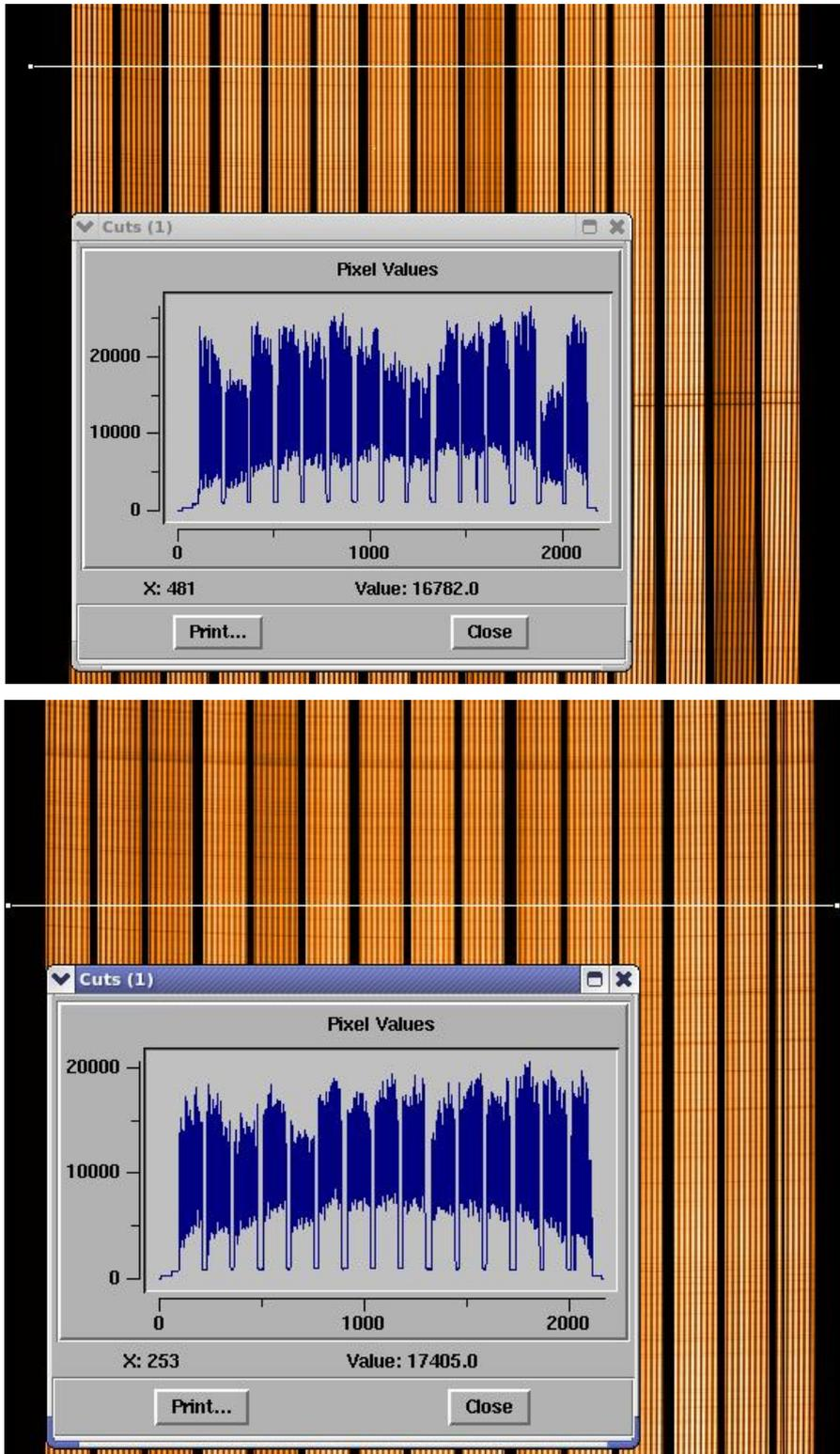
Figure 24: Raw GIRAFFE IFU images of the solar spectrum on plate 1 (top) and plate 2 (bottom). Variations in the IFU responses are clear.
