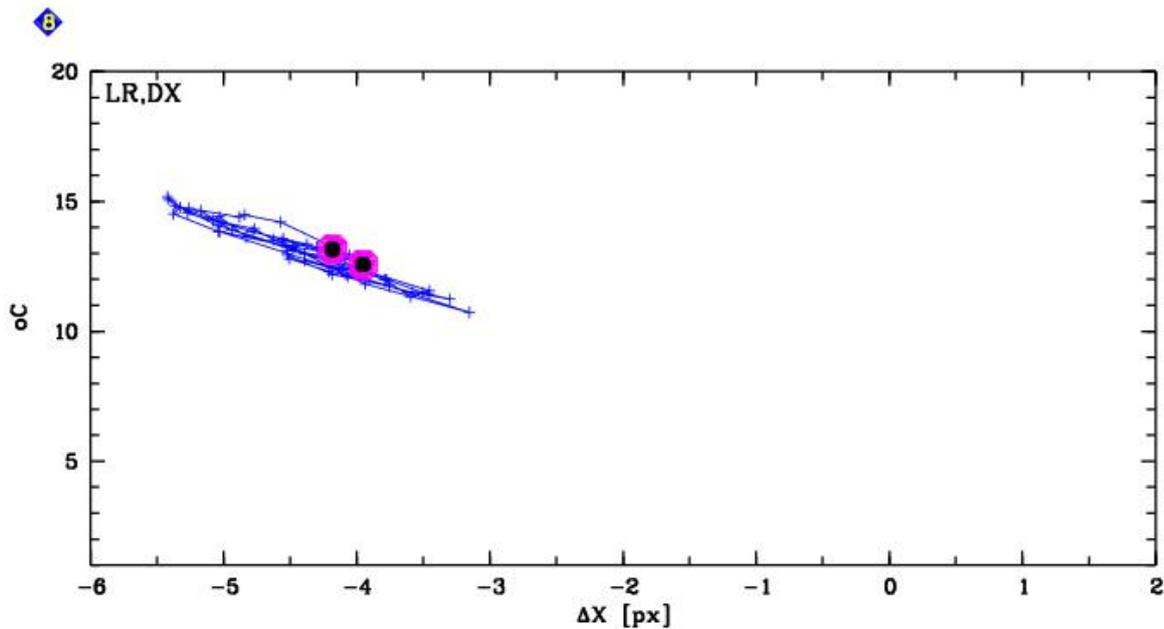
Figure 30: Shift of GIRAFFE X-axis with temperature in late 2008/early 2009. Calibrations are taken the day after the science and the temperatures are inspected so that they are within 1.5 C.
