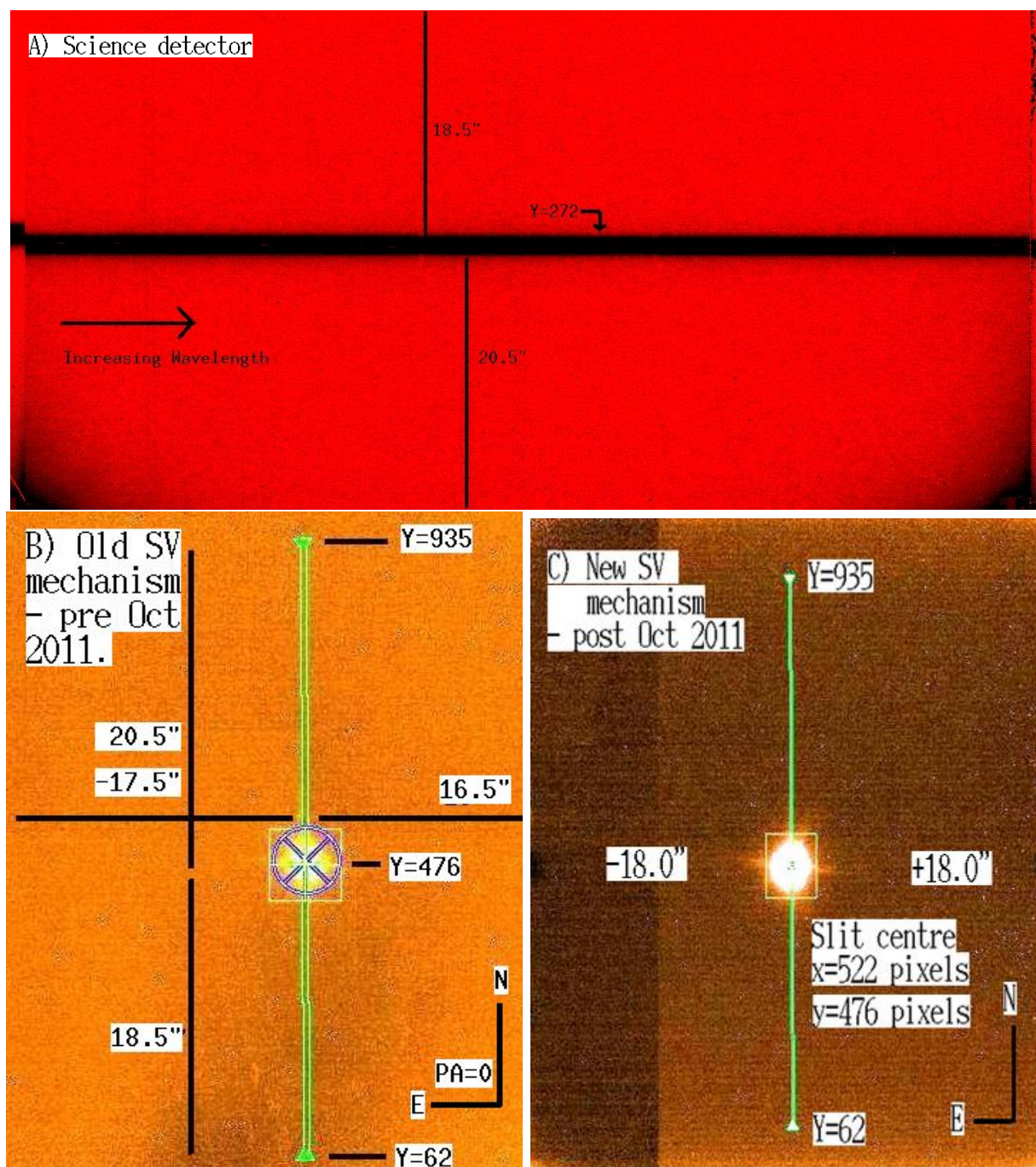
Figure 24: Illustration of the geometry of the science (A) and slit viewer detector (B,C) for a PA of 0 deg on sky. Two SV images are shown; (B) is with the old slit unit and (C) with the new slit. On the science detector, North is to the bottom and East to the left, while North is to the top and East to the left on the slit viewer detector. The centering position of the science target in the SV detector is the center of the slit in x and pixel y = 476 along the slit. This position corresponds to pixel y \approx 293 on the science mosaic; the exact value depends on the detector and the wavelength setting. With the templates CRIRES_spec_obs_AutoNodOnSlit and CRIRES_spec_obs_SpectroAstrometry , nodding is done symmetrically along the slit around the centering position. For nodding position A, the image of the target appears at larger y values on the slit-viewer and lower y value on the science detector, at half the nod throw from the centering position. In other words, for a PA of 0 deg, the telescope position at nodding position A is South of the centering position. Conversely, for nodding position B, the image of the target appears at smaller y values on the slit-viewer and larger y value on the science detector. On the science detector, wavelengths increase from left to right.
