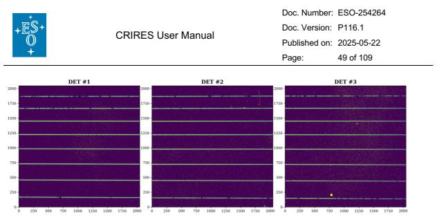
Figure 36: Illustration of the science detectors mosaic (H1582 setting).
