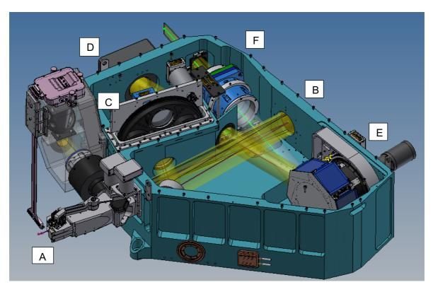
Figure 4: Top view of the new CRIRES fore-optics assembly
