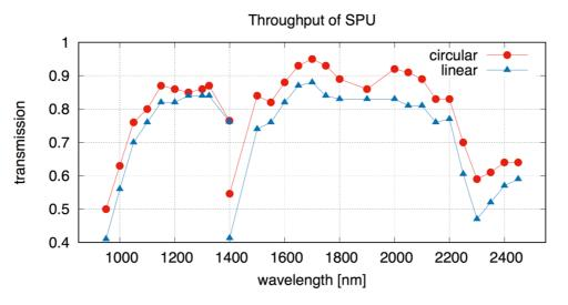
Figure 29: Measurements of the throughput of the Spectro-Polarimetry Unit (SPU).
