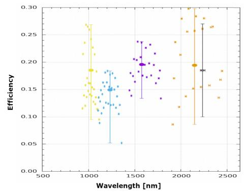
Figure 37: Efficiency of CRIRES measured using a blackbody source in the lab in the YJHK bands.
