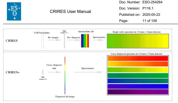
Figure 3: Schematic diagram summarizing the differences between oCRIRES and CRIRES after the upgrade
