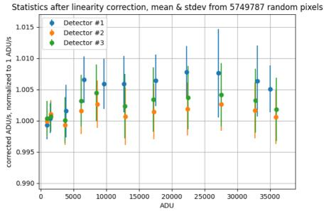
Figure 27: Normalized ADU/s as measured from the frames corrected for non-linearity. For the three detectors, the median over the bins in ADU-level is given. A value of 1.005 on the *y*-axis corresponds to 0.5% inaccuracy.
