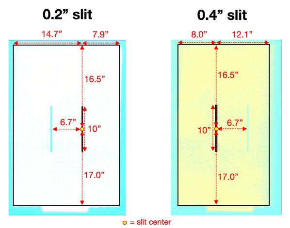
Figure 28: Sketch of the SV detector for position angle of 0 degrees in the SKY derotator mode (§6.3.5). In this setting, North is up and East towards the left. Note that the field-of-view (FoV) of the unvignetted SV detector depends on the slit used. For both slits, the footprint of the unused slit is located parallel to the used slit (the 0.4" slit is located 6.7" to the left with respect to the 0.2" slit).
