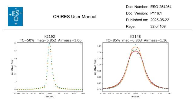
Figure 22: AO mode PSF profiles for different Turbulence Categories (30%, 50% and 85%) in the H- and K-bands (note the different scales of the y-axes).
