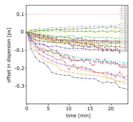
Figure 34: Relative drift in pixel in main dispersion during 24 min after the completion of the metrology. The offset is relative to the position at the completion of metrology.
