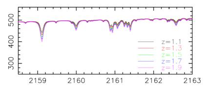
Figure 41: Effect of changes in airmass on PWV absorption produced by the CRIRES ETC.
