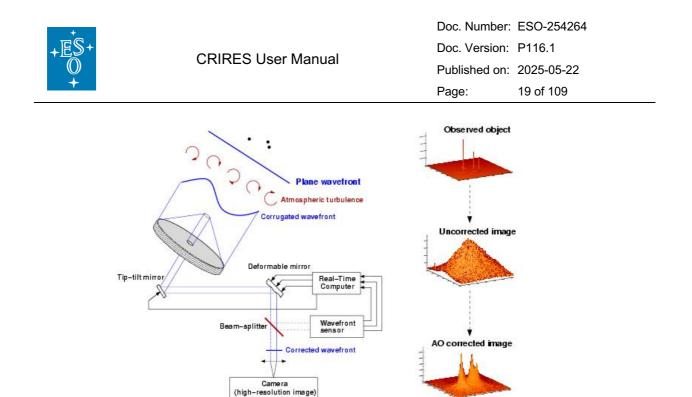
Figure 10: Principle of Adaptive Optics. Note that in practice, and contrary to this schematic design, CRIRES has no dedicated tip-tilt mirror, but performs low- and high-order correction with a single deformable mirror mounted on a tip-tilt stage (see Figure 12).
