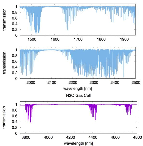
Figure 17: Absorption line spectrum of the new short gas cell (SGC) in the H and K bands (top) and the  $N_2O$  gas cell in the L and M bands (bottom). The FTS scan of both cells is provided on the CRIRES webpages under 'Tools'.
