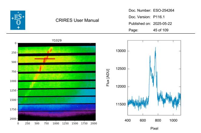
Figure 33. <u>Left:</u> Flat-field exposure exhibiting the optical ghost on Detector 2 in the Y1029 wavelength setting. Note that the ticks correspond to detector pixel. The brown horizontal line depicts the area of the flux distribution shown in the <u>right panel</u>.
