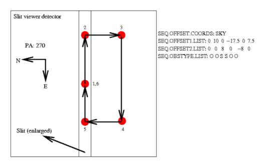
Figure 44: Illustration showing the apparent locations of the targets <u>relative to the slit centre</u>, as seen on the SV detector for the given parameters in the SKY coordinate offsets in units of arcsec. If the telescope moves North, the target moves South relative to the slit centre.
