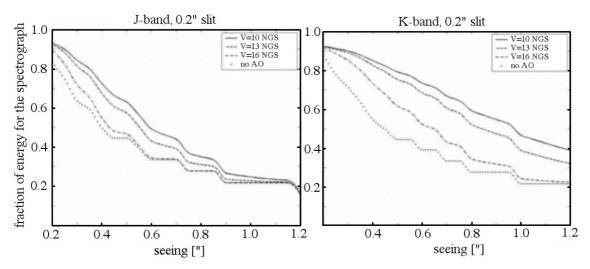
Figure 20: The fraction of energy available for the spectrograph in a 0.2" slit as a function of the optical seeing is shown for the J (left) and K (right) band for NGS of V=10, 12, 16 mag and without AO correction. For reference, please consult the ETC.
