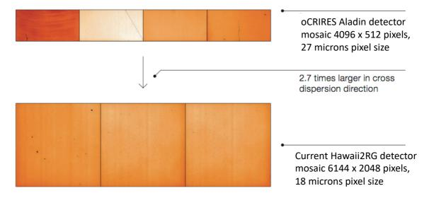
Figure 6: The original CRIRES detector mosaic (upper image) compared to the new detectors with an increase of a factor of 2.7 in the cross-dispersion direction (lower image).
