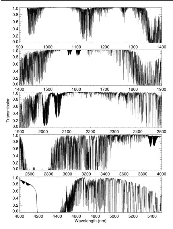
Figure 38: Atmospheric transmission from 900-5500nm computed by PCLnWin/HITRAN for Paranal atmosphere, PWV = 2.5mm, at zenith and smoothed to a resolution of  $\lambda/\Delta\lambda$  = 10,000.
