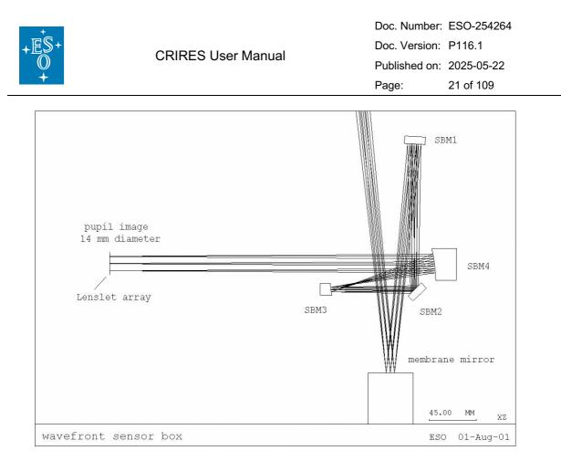
Figure 13: The optical path of the wavefront sensor box.
