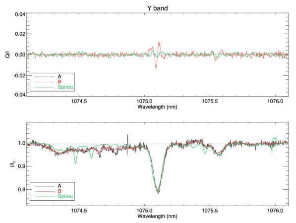
Figure 31: The Stokes Q polarization is shown for the star Gamma Equ (H=4.18) at both nodding positions A and B, taken with the 0.2" wide slit; for comparison, we show the performance of the Spirou spectrograph (green line). The exposure time of one exposure was DIT x NDIT = 20s x 4. Note that a total of four exposures were taken at each nodding position, with the polarimeter rotator angles at 0, 90, 180 and 270 degrees (see §6.3.7).
