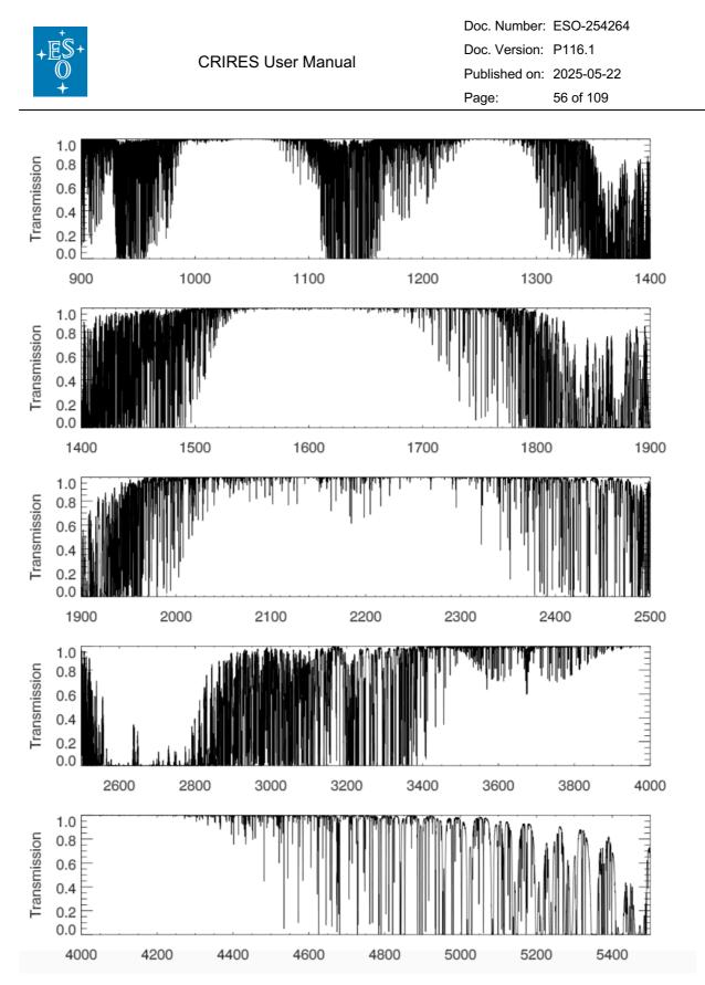
Figure 39: PWV sensitive atmospheric transmission from 900-5500nm computed with RFM/HITRAN for Paranal atmosphere, PWV=2.5 mm at zenith at resolution of  $\lambda/\Delta\lambda$  = 10,000.
