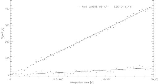
Figure 25: Dark current of detector #3 measured in K band
