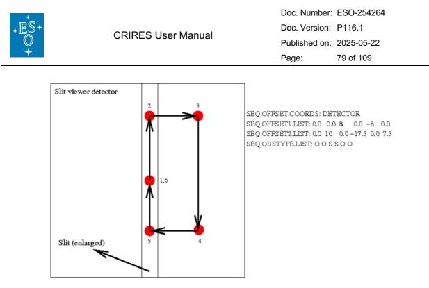
Figure 43: Illustration showing the apparent locations of the target <u>relative to the slit centre</u>, as seen from the SV detector for the given parameters, for the case of DETECTOR coordinate offsets. Offsets in X are perpendicular to the slit, while offsets in Y are always parallel to the slit. All motions are made in units of arcsec.
