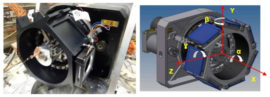
Figure 5: Grating wheel design with locking mechanism and build prototype
