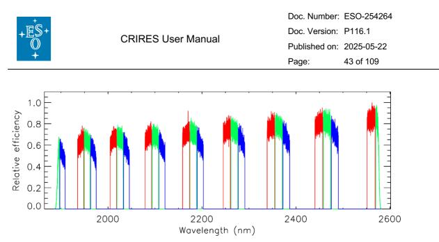
Figure 32: A 1D-extraction of the flat-field image indicating the spectral coverage achieved for a single echelle setting, obtained in a single exposure (K-band, echelle angle=65.5). The three different detectors are colour-coded differently.
