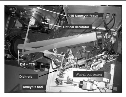
Figure 11: Top view of the warm optics of the MACAO-CRIRES system. From f/15 Nasmyth focus and after the optical derotator, one notices the deformable mirror and the tip-tilt mount assembly. Light enters from the dichroic to the cold and warm part of the instrument. On the right the wavefront sensor and some analysis tools are visible.
