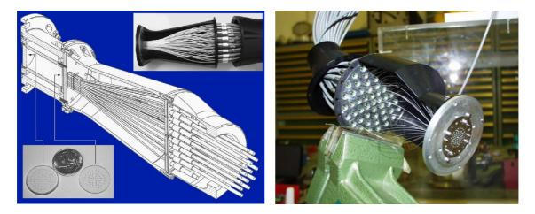
Figure 14: Front-end assembly of the 60 fiber bundle which guide the light to the sensors.
