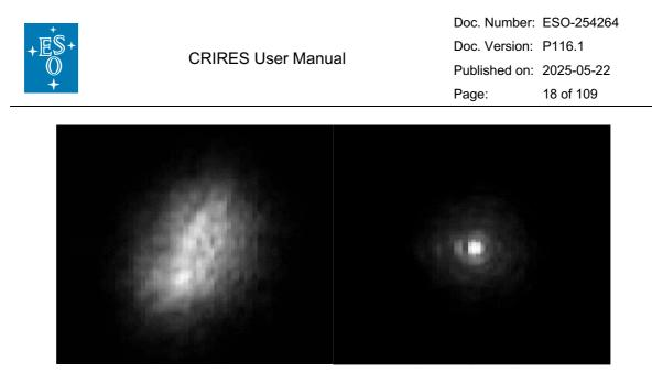
Figure 9: PSF without (left) and with (right) MACAO correction. Images have been taken in the lab using a turbulence generator.
