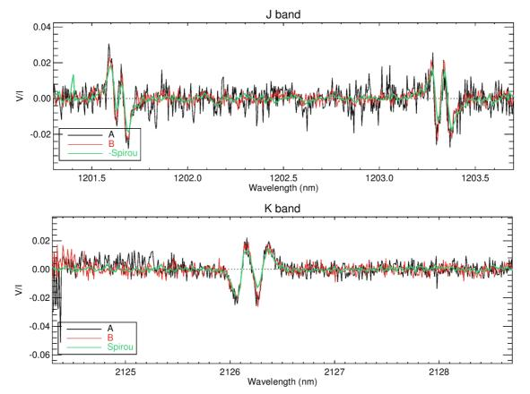
Figure 30. The Stokes V polarization is shown for the star Gamma Equ (H=4.18) at both nodding positions A and B, taken with the 0.2" wide slit; for comparison, we show the performance of the Spirou spectrograph. The upper panel depicts a wavelength chunk in the J-band, while the lower panel one in the K-band. The exposure time of one exposure
