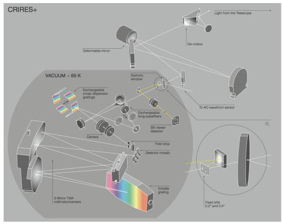
Figure 1: Optical layout of CRIRES
