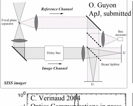
**SISS (Synchronous Interferometric Speckle Subtraction)** = Specles are coherent with the central source, Planets are not!
