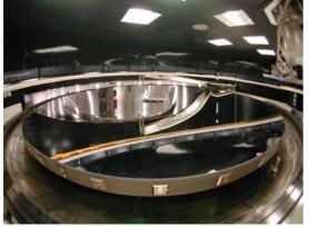
Figure 5: Primary mirror right after aluminization
