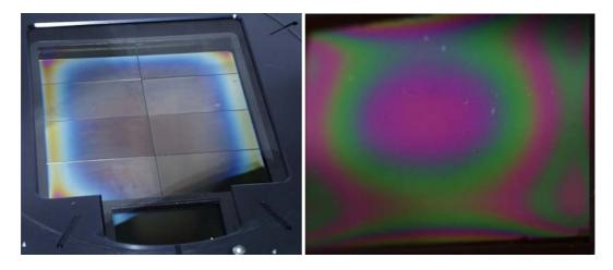
Figure 8: Contaminated CCD chips
