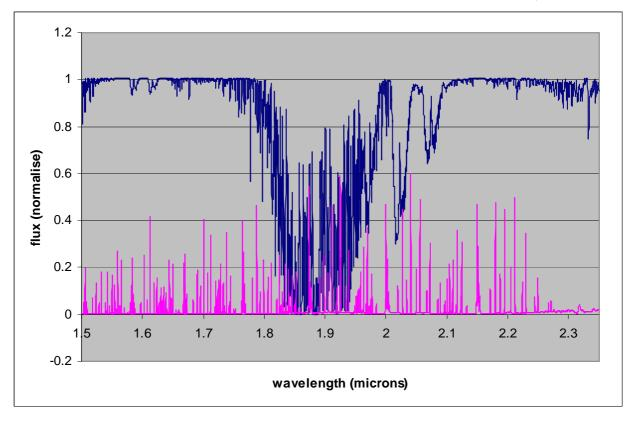
Figure 4: Simulated transmission and OH emission spectrum for the HK grating. The OH units are arbitrary, scaled to be plotted alongside the transmission.
