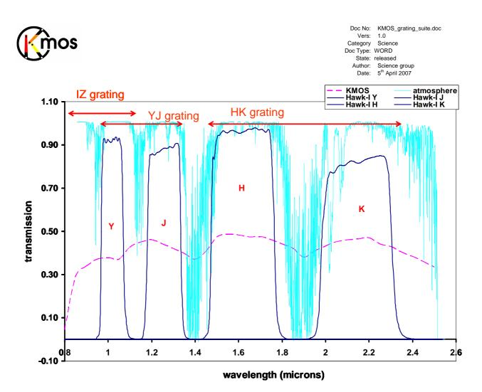
Figure 5 Hawk-I filters and KMOS wide (IZ, ZY, HK) gratings shown in red for comparison. The KMOS transmission curve includes filters and the grating efficiency curves for the original grating suite. The  $0.8\mu$ m transmission will be improved with optimisation of the blocking before FDR. The detector QE is not included.
