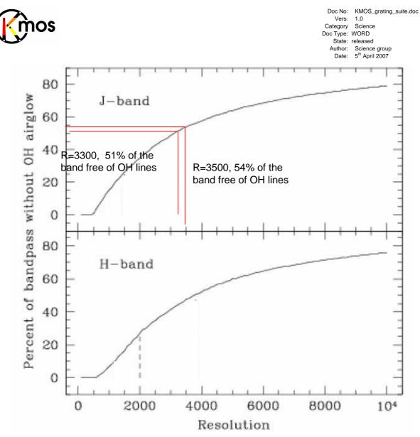
Figure 3: From Depoy & Martini, the effect of resolution on OH line coverage.
