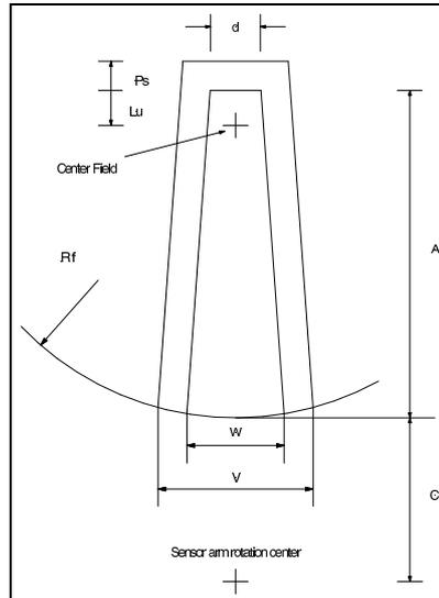
Figure 7: Guide-probe shadow in the Cassegrain focal plane. See table 5 for the dimensions.
