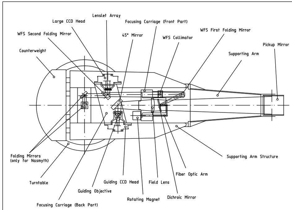
Figure 6: Schematic view of the adapter sensor arm.
