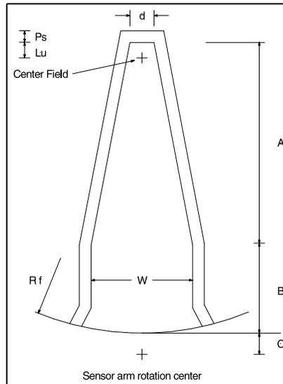
Figure 8: Guide-probe shadow in the Nasmyth focal plane. See table 5 for the dimensions.
