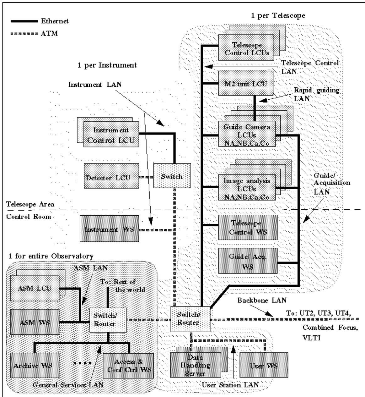
Figure 9: Logical lay-out of the VLT LANs
