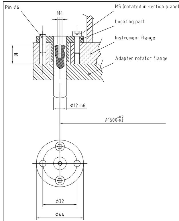
Figure 10: Proposed design for a reference pin adjustment device
