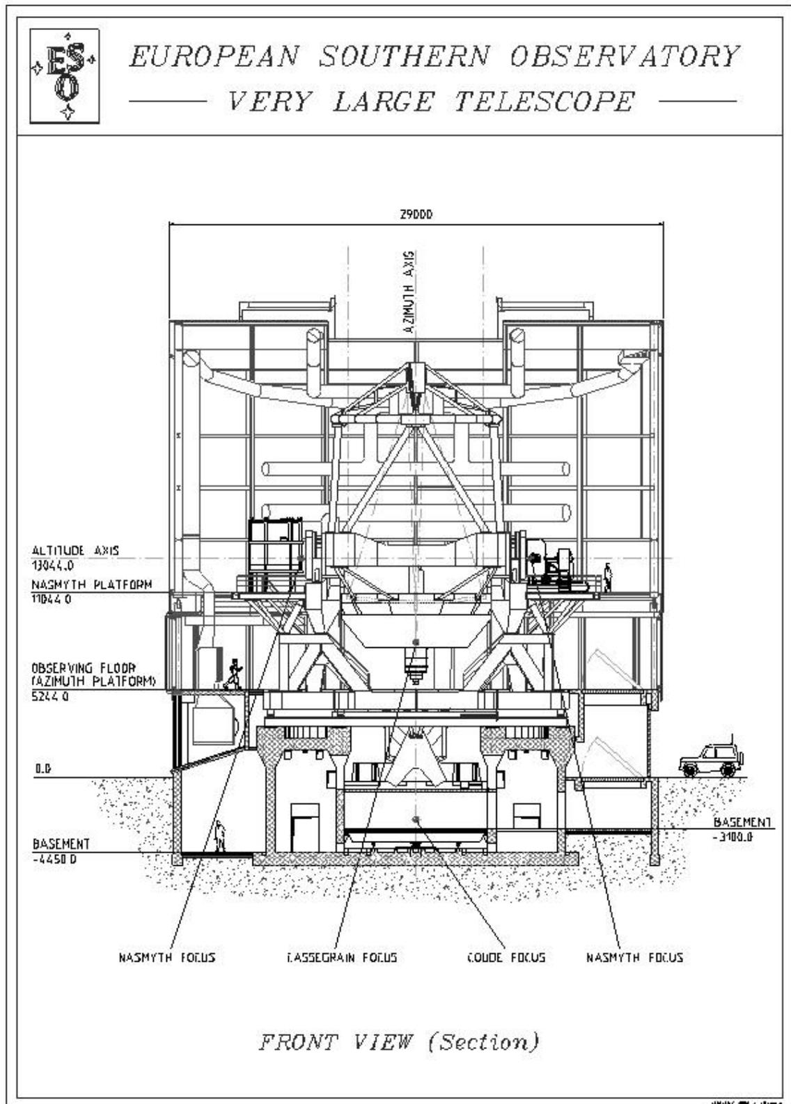
Figure 3: Front view of a Unit Telescope
