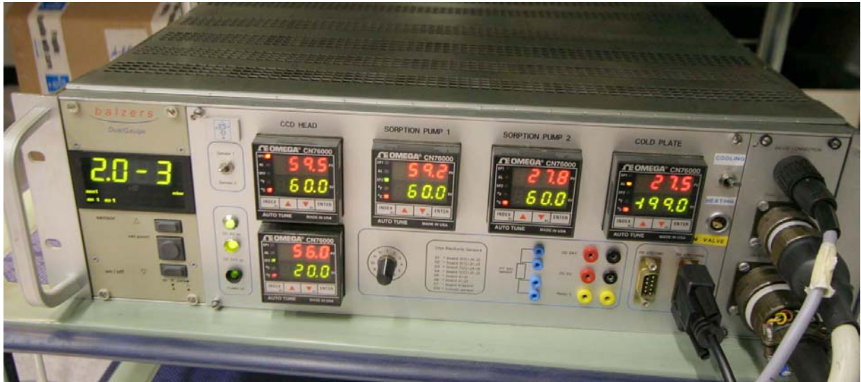
Figure 1: CRYMAC used for baking of the CCDs and the sorption pump(s) as preparation for the synthetic air treatment process
