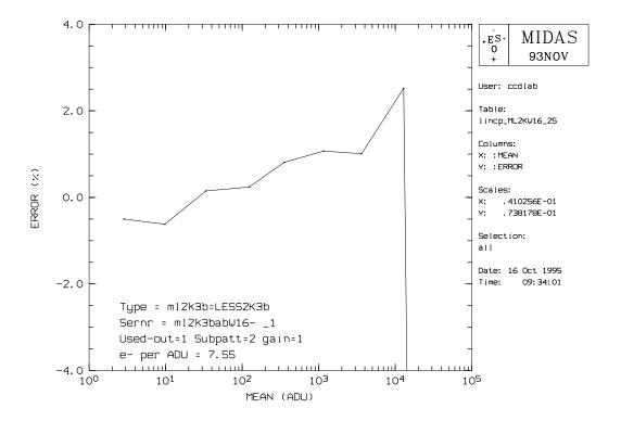
Figure 2: Linearity Measurement with amplifier 2
