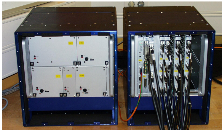
Figure 3 - FIERA power supply and detector head box
