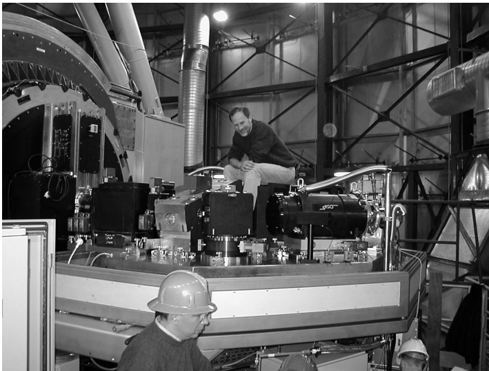
Figure 1 - UVES instrument during installation at the telescope
