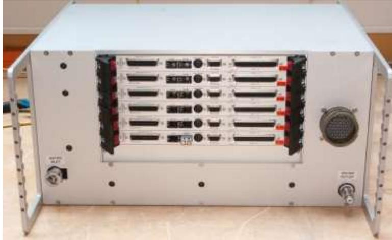
Figure 3. 6-slot NGC detector front-end
