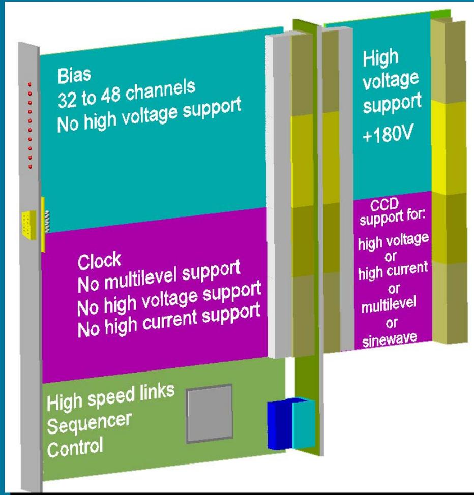
The platform supports **add-ons** for special detectors and does not limit future design of **dedicated boards**
