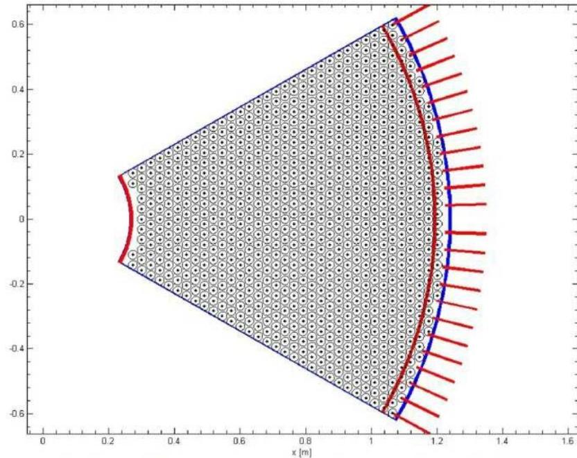
Fig. 3: Mirror shell layout with actuator pattern
